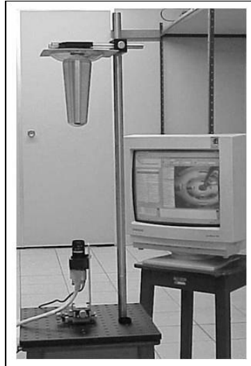
Figure 6. Picture of the omnidirectional stereo system.
