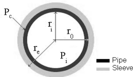
Figure 1: Pipe and sleeve with internal pressure.
