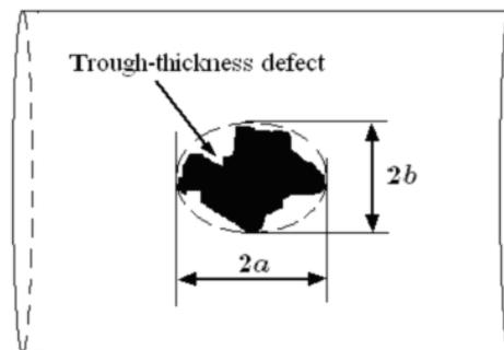
Figure 3: Defect sizing.
