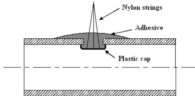
Figure 5: Plastic cap to avoid adhesive spilling.
