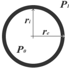
Figure 12: Pipe under external and internal pressure.
