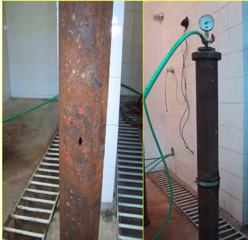
Figure 11: 3,5" diameter, schedule 20, 1000 mm length pipe with real corrosion defect before and after repair.
