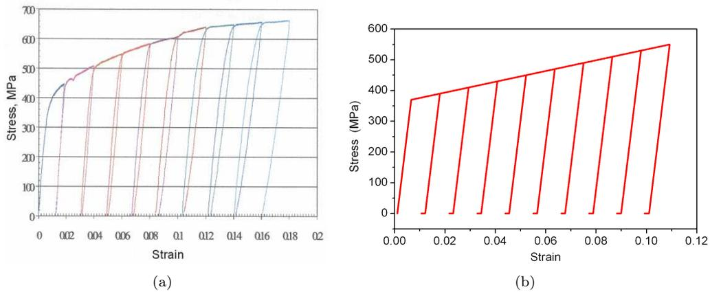
Figure 5: Stress-strain diagram for qualitative comparison between numerical results provided by the model and experimental results by [24] for cyclic test to verify plastic-phase transformation coupling. (a) Experimental result; (b) Numerical result.
