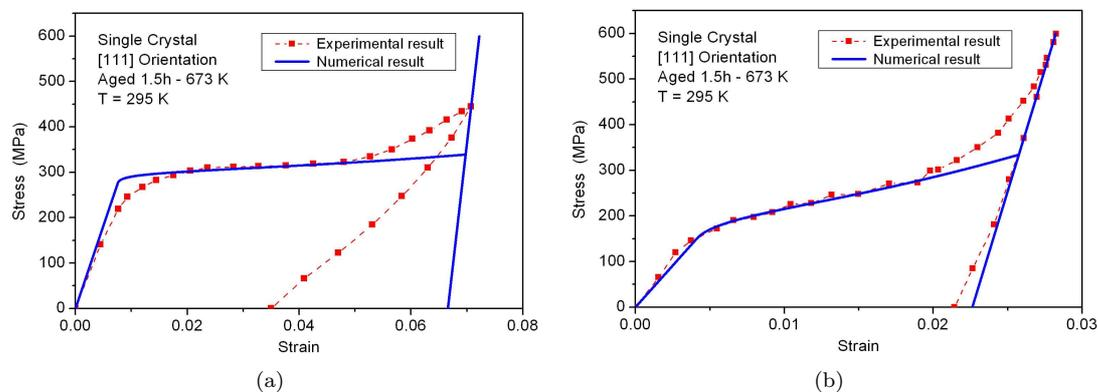
Figure 4: Comparison between numerical results provided by the model and experimental results by [23] for tensile-compressive asymmetry. (a) Tensile test; (b) Compressive test.
