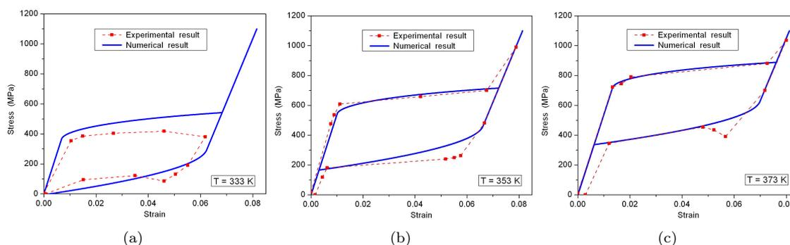
Figure 1: Comparison between numerical results provided by the model (without considering TRIP phenomenon) and experimental results by [20] for pseudoelastic behavior for three different temperatures. (a)  $T = 333$  K; (b)  $T = 353$  K and (c)  $T = 373$  K.
