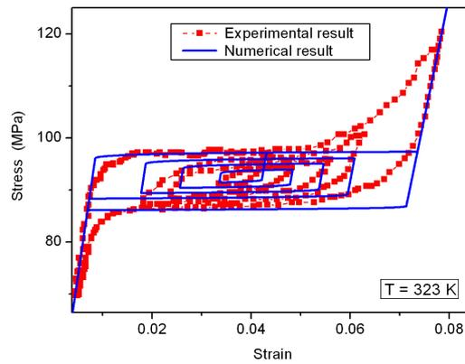
Figure 3: Comparison between numerical result provided by the model and experimental result by [22] for pseudoelastic subloops.
