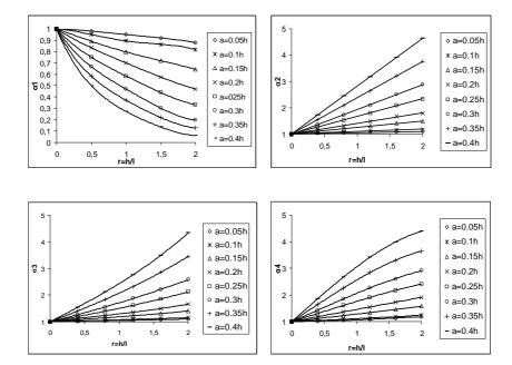
Figure 1: Coefficient value for the evaluation of the stiffness matrix modeling the cracked element when the crack is open. [6]
