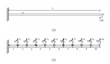
Figure 5: Cantilever beam: (a) for numerical application (b) representation for finite element
