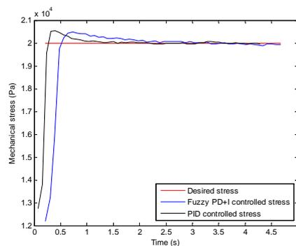
Figure 8. Comparison between PID and fuzzy controllers.
