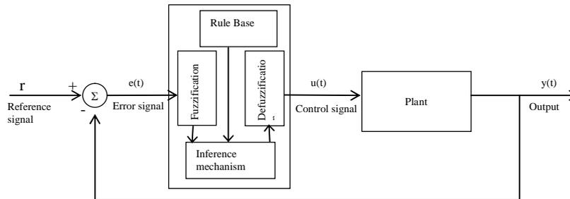
Figure 2. Fuzzy controller inserted in the control loop
