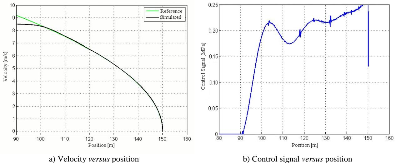
Figure 6. Braking action with transported mass of 13360kg (Simulation).
