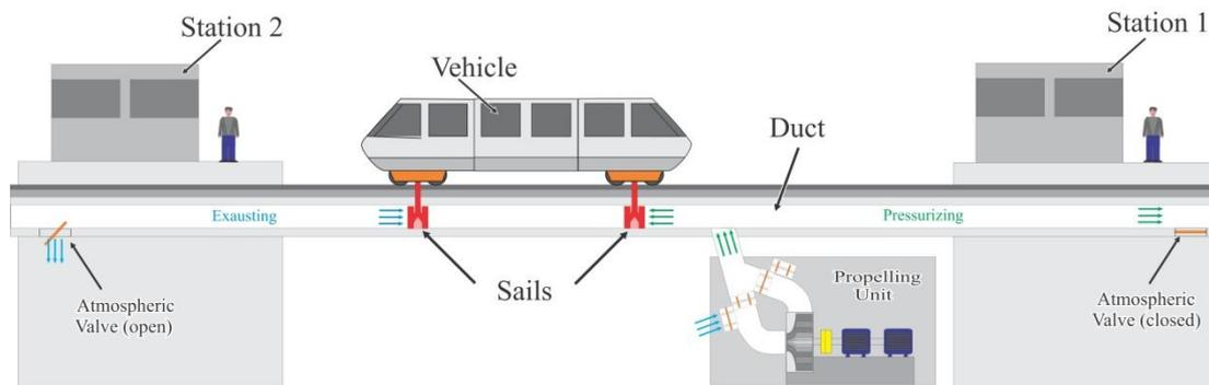
Figure 1. Schematic view of the Aeromovel system.
