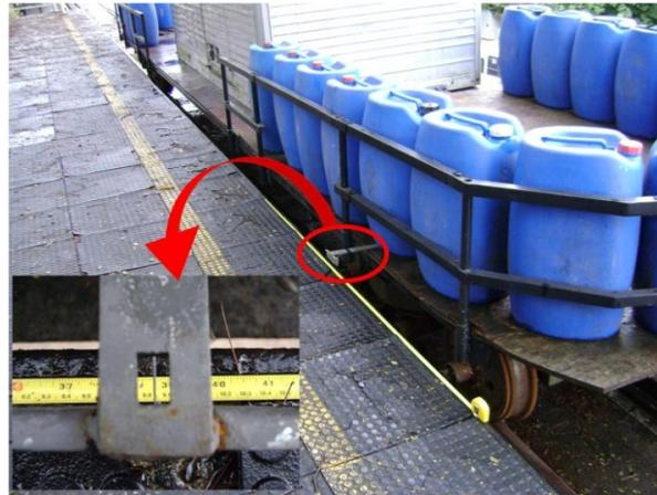
Figure 7. Method to measure the brake error.
