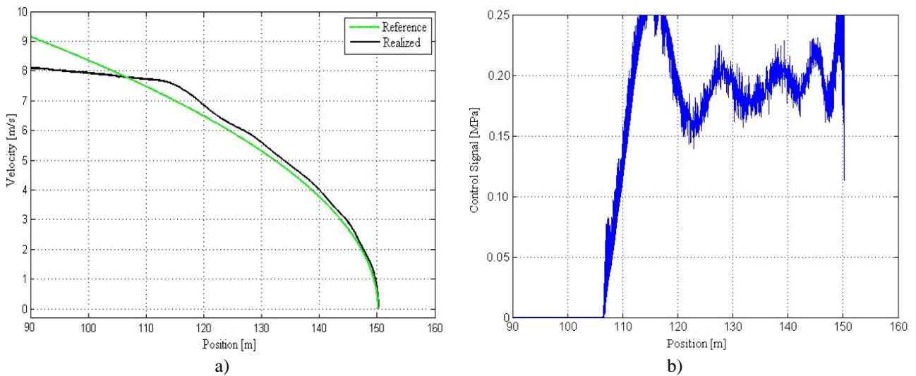
Figure 9. Braking action with transported mass of 13360kg (Experiments).
