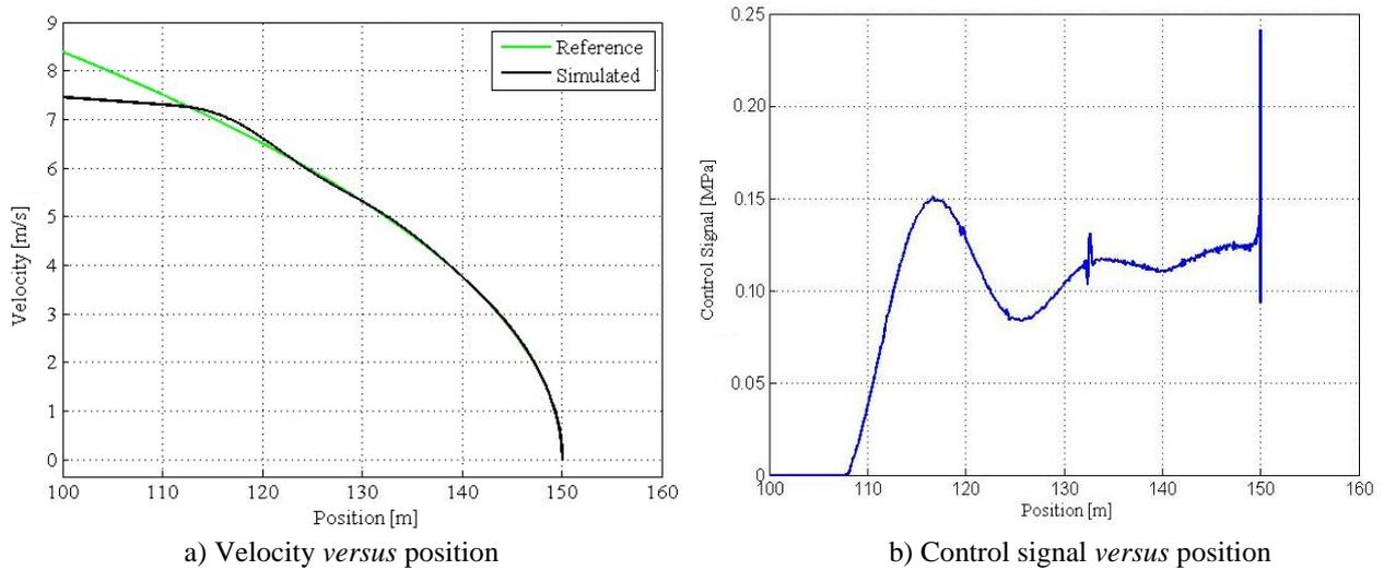
Figure 5. Braking action with transported mass of 7735kg (Simulation).
