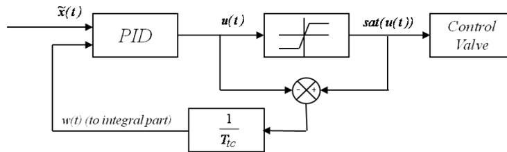
Figure 4. Block diagram of anti-wind-up scheme.
