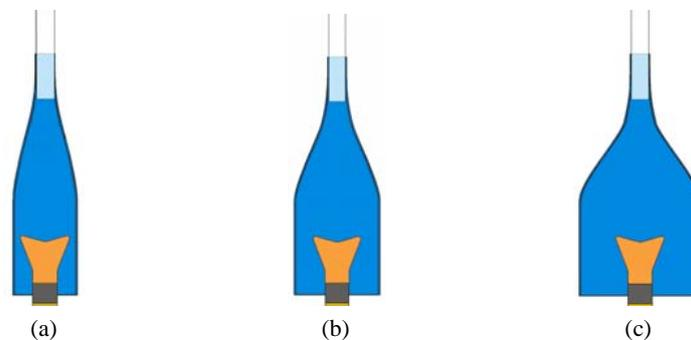
Figure 8. Pump channels tested. (a) width = 60 mm; (b) width = 80 mm; (c) width = 100 mm
