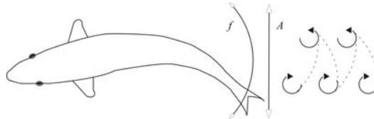
Figure 1. Vortex street wake generated by a fish swimming
