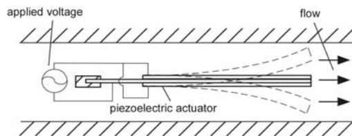
Figure 2. Piezoelectric pump scheme
