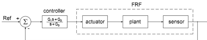
Figure 1. Block diagram of the closed loop system.
