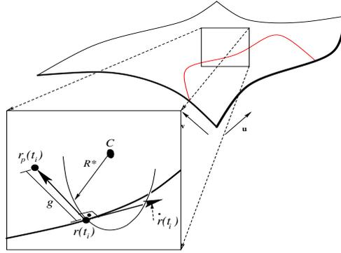
Figure 6. Geometric relationships to compute a parallel path.
