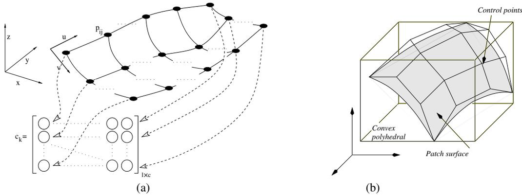
Figure 1. Net of points, its matrix arrangement and Bezier convexity property.
