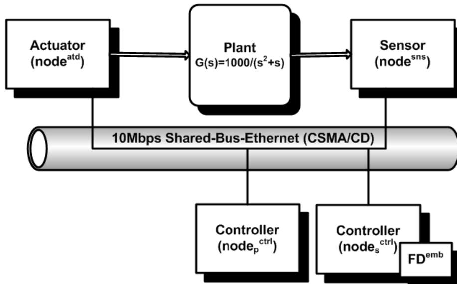
Figure 1. Distributed control system with failure detector
