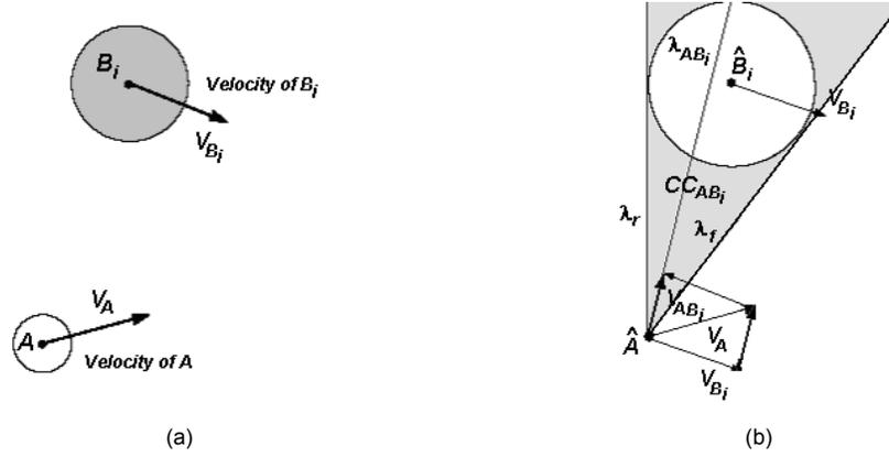
Figure 2. Velocity Obstacle Approach: (a) the robot is represented by A and the obstacle, by B<sub>i</sub>. (b) Collision Cone between  $\hat{A}$  and  $\hat{B}_i$ :  $CC_{AB_i}$ .
