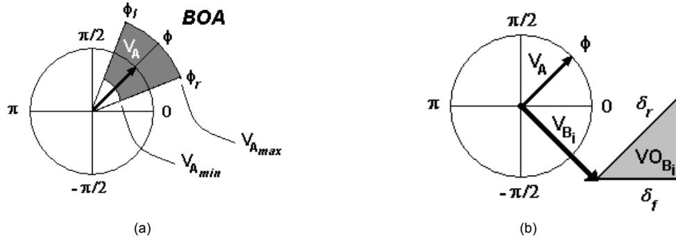
Figure 6. *BOA* Procedure: (a) the circle of radius  $\|V_A\|$  represents the velocity space and the dark gray area limited by  $\phi_l$ ,  $\phi_r$ ,  $V_{Amax}$ , and  $V_{Amin}$  represents the set of *reachable velocities*. (b) The use of  $VO_{B_i}$  to calculate the *dangerous velocities*.
