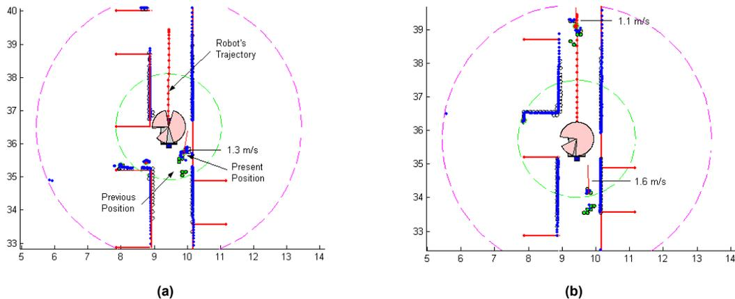
Figure 11. *BOA* Procedure: illustration of the *DVD* sets (salmon areas), laser data (blue dots), environment map (red lines) a person walking close to MOPS at 1.3 m/s (a) and 2 persons walking close to MOPS at 1.1 m/s and 1.6 m/s (b).
