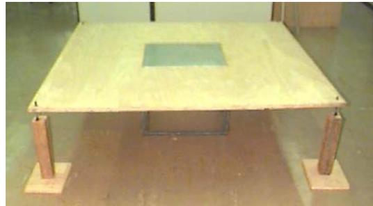
Figure 8. The plate mounted on a finite baffle.
