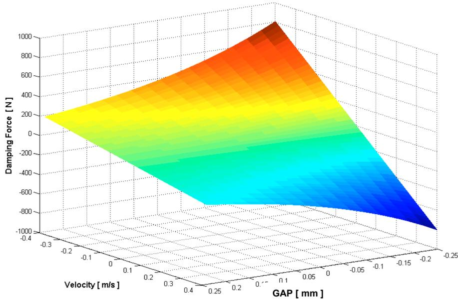
Figure 9. Analitical model for Damping Forces.
