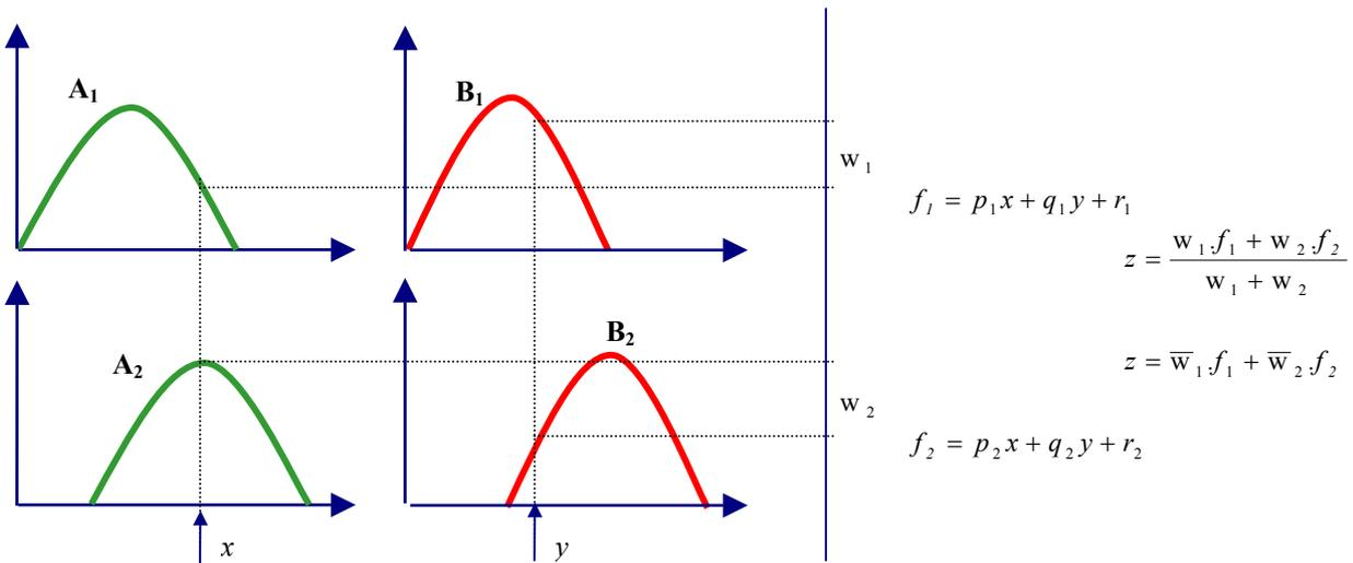
Figure 10. First order Sugeno fuzzy system with two inputs and one output.
