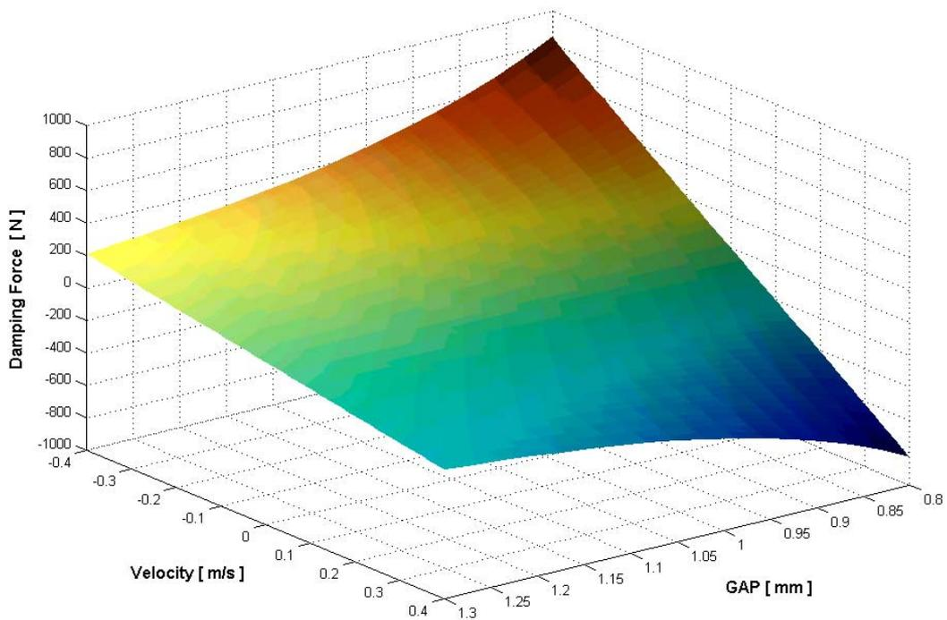
Figure 7. Finite element simulations of the damping force
