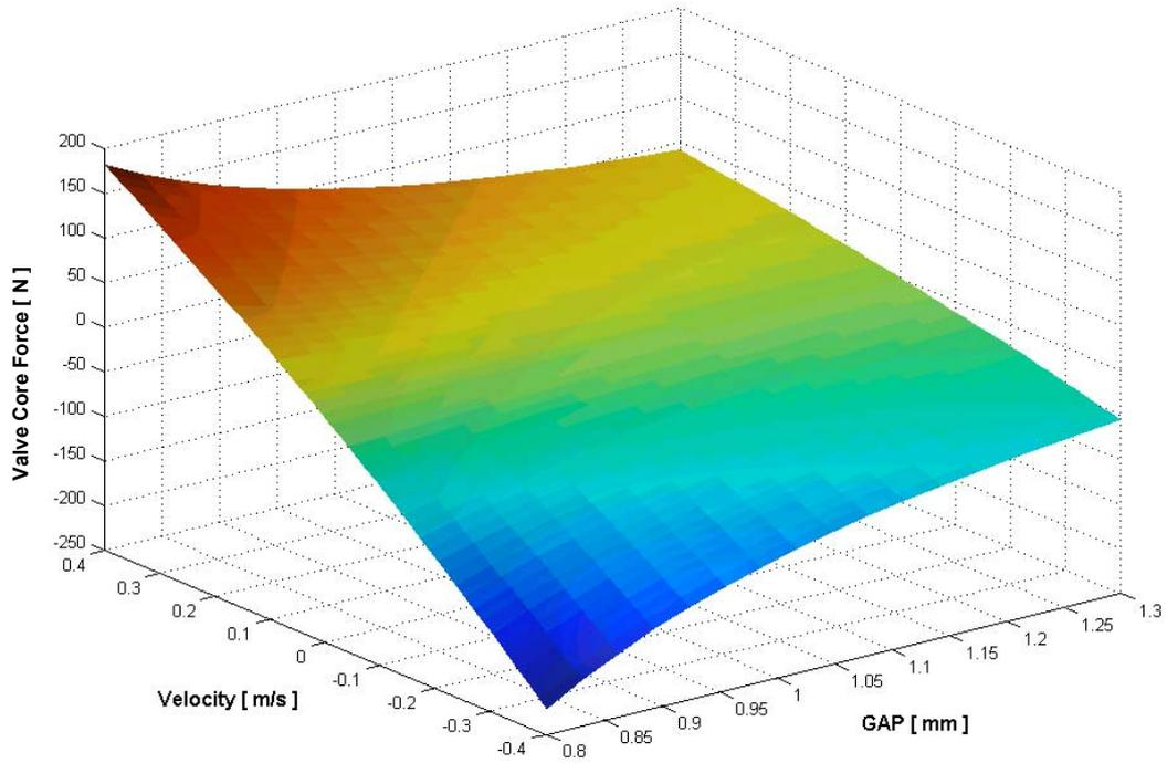
Figure 6. Finite element simulations of the forces at the valve core.
