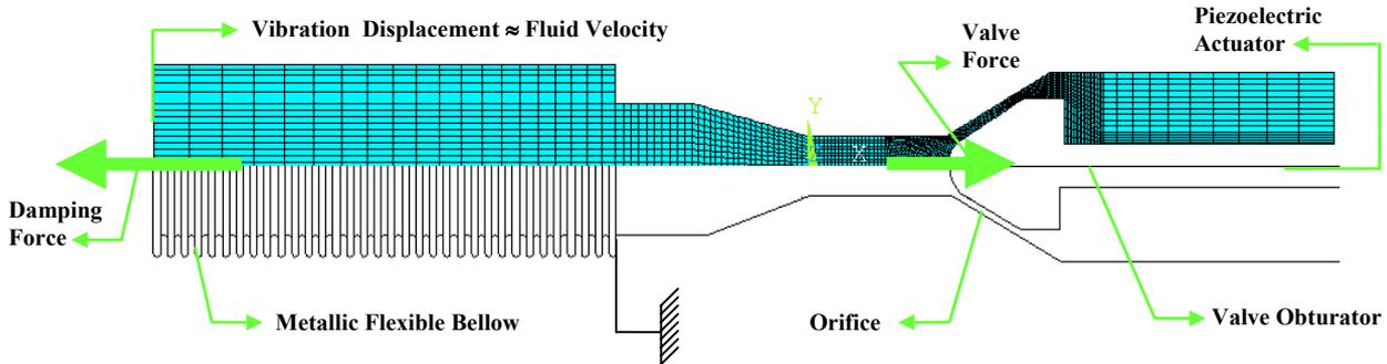
Figure 2. Finite element axi-symmetric model of the hydraulic circuit.
