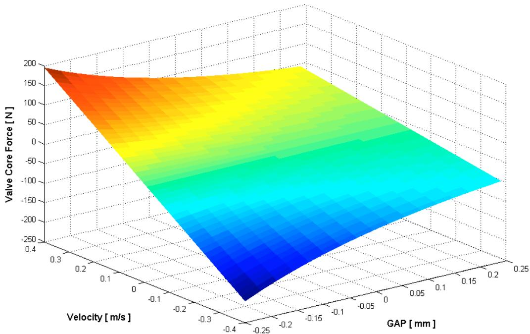
Figure 8. Analitical model for the Force at the valve core..
