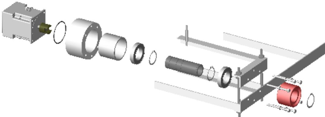
Figure 6. Mechanical parts of the actuator module.
