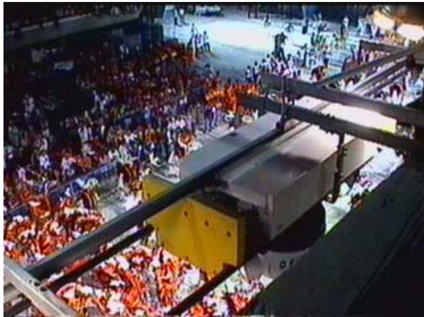
Figure 24. Photo of the telerobotic trolley in operation.
