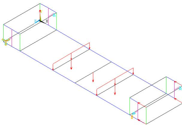
Figure 22. FEM of the trolley with external forces.
