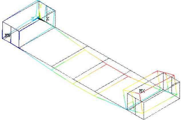
Figure 23. Trolley nodal displacements of Fig. (22).
