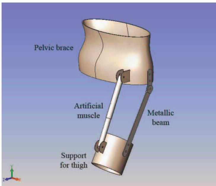
Figure 1 – Project of the orthosis parts with the artificial muscle (Exoskeleton).
