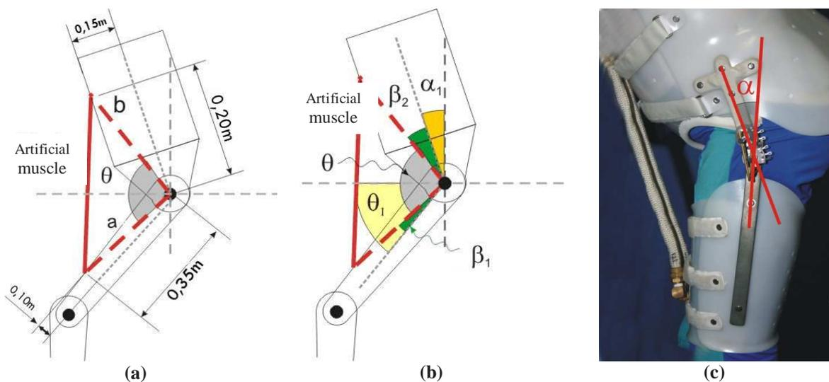
Figure 4 – (a) Determination of the muscle length, (b) Determination of the angle (c) Patient using the orthosis.
