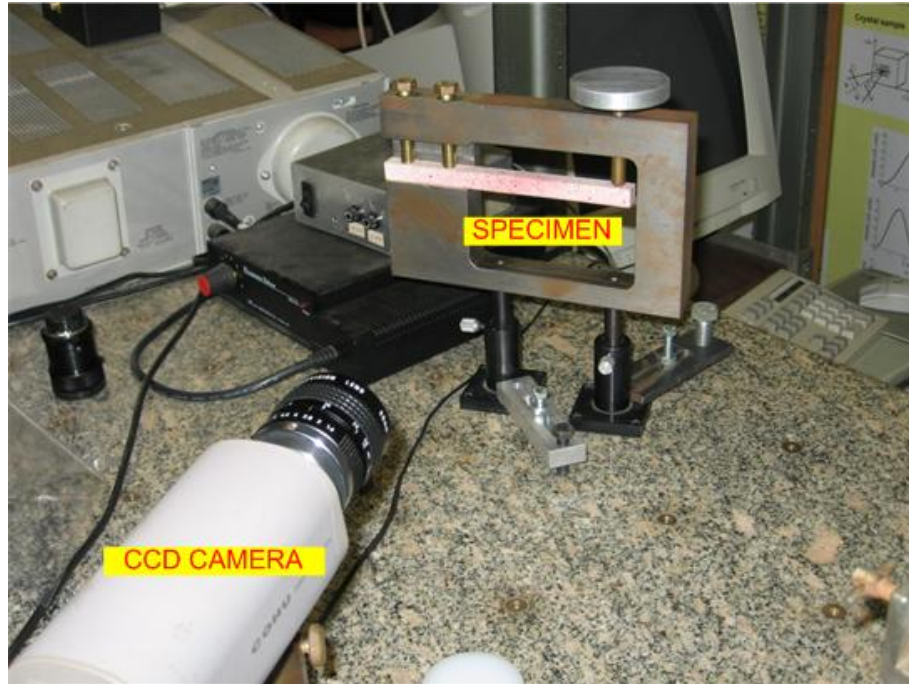
Figure 3. Experimental arrangement of DIC method.
