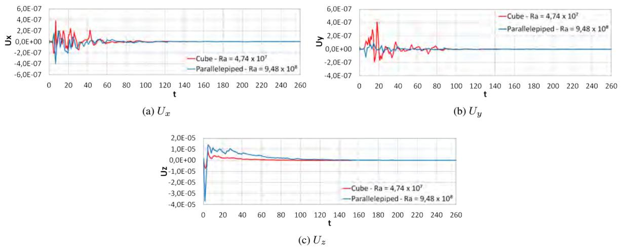
Figure 8: Components of Average Velocity with Time Varying.
