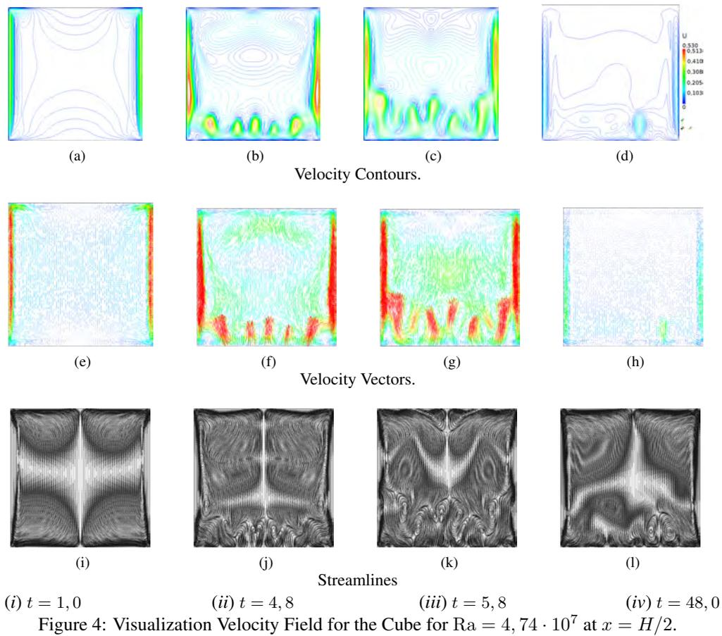
Figure 4: Visualization Velocity Field for the Cube for  $Ra = 4,74 \cdot 10^7$  at  $x = H/2$ .
