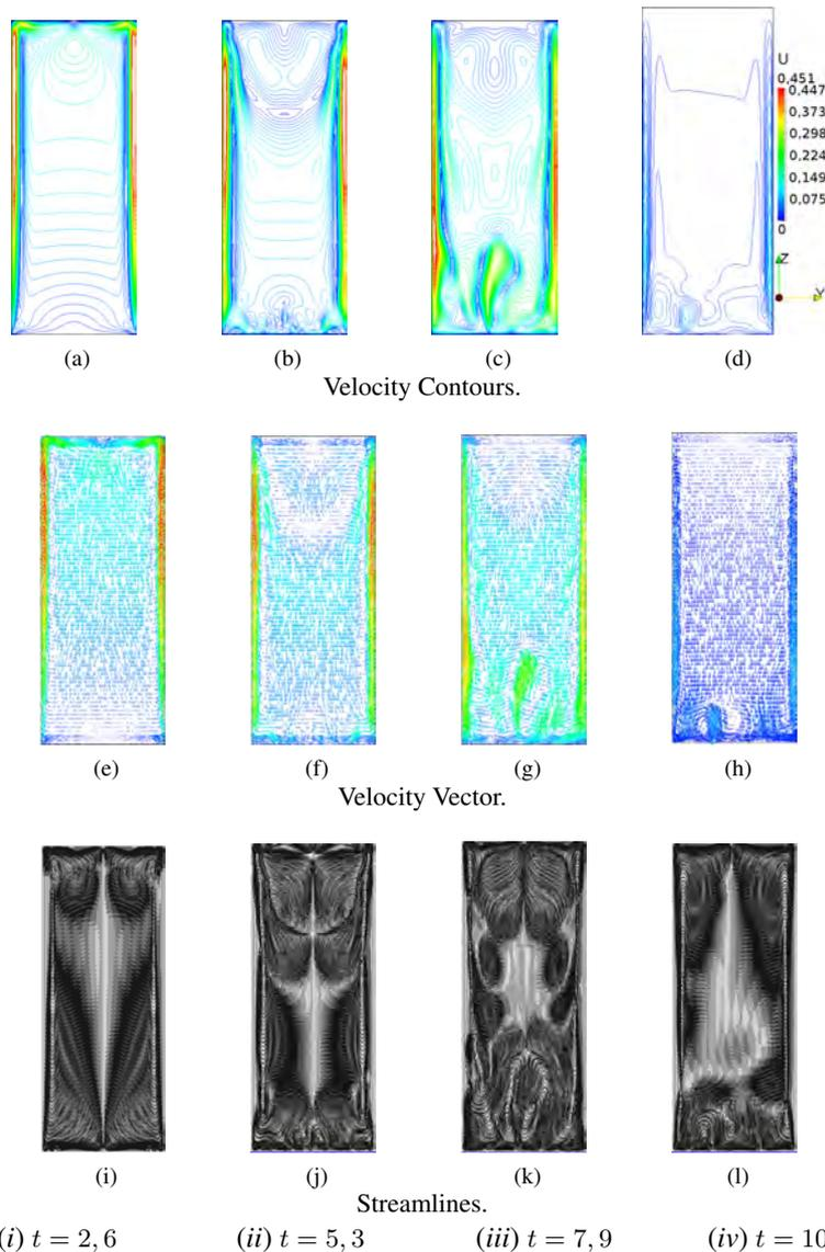
Figure 6: Visualization Velocity Field for the Parallelepiped for  $Ra = 9,48 \cdot 10^8$  at  $x = H/2$ .
