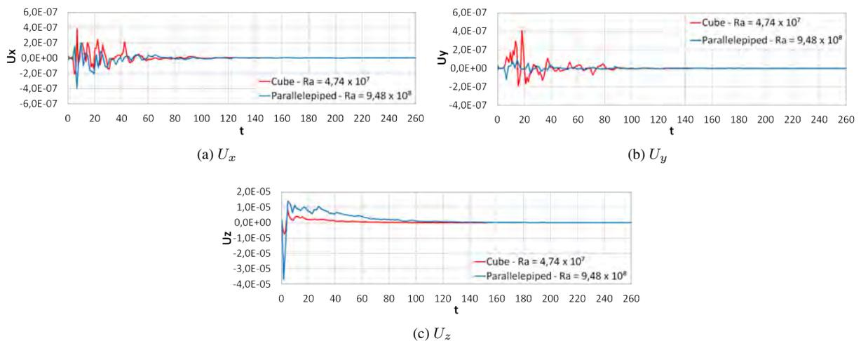
Figure 8: Components of Average Velocity with Time Varying.
