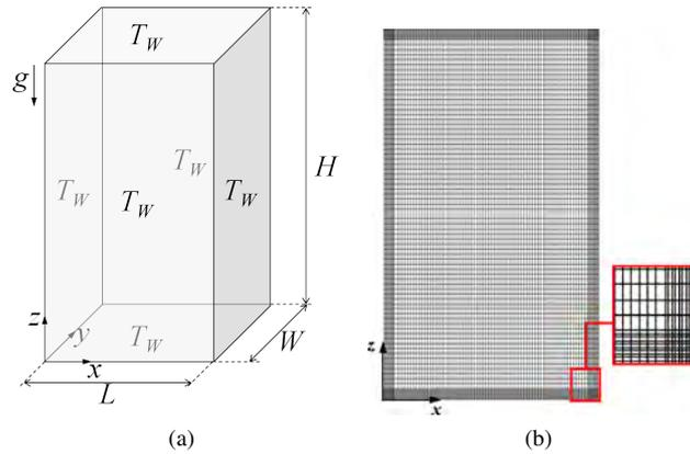
Figure 1: Cavity: (a) Boundary Conditions; (b) Mesh Detail.
