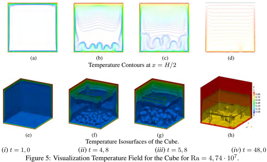
Figure 5: Visualization Temperature Field for the Cube for  $Ra = 4,74 \cdot 10^7$ .
