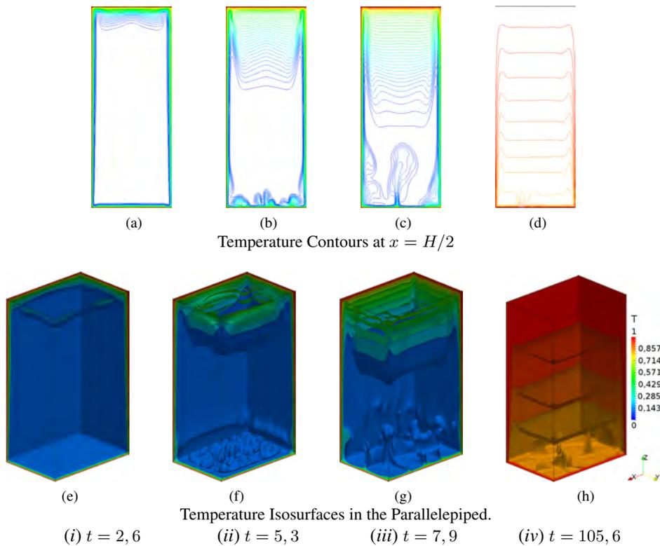
Figure 7: Visualization Temperature Field for the Parallelepiped for  $Ra = 9,48 \cdot 10^8$ .
