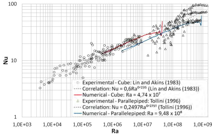
Figure 3: Comparison of Nusselt *versus* Rayleigh with experimental data.
