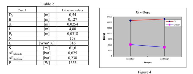
In this case while the capital cost increased by 4.4% owing to an increase of tubes number, which compensates their length reduction leading to a net increase of the heat exchanger surface, the total cost was reduced of about 2.52 % thanks to a 24.13% reduction of discounted operating costs caused by a reduction of tube side pressure drop.
