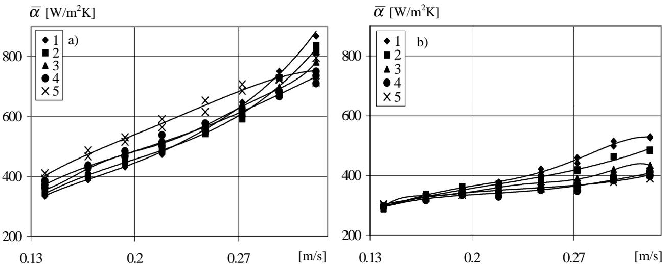
Figure 5. Heat transfer of the middle line of the tube bundle: a)  $\beta = 0.996$ ; b)  $\beta = 0.998$ ; 1, 2, 3, 4, 5 – B1, B2, B3, B4, B5 tube correspondingly.
