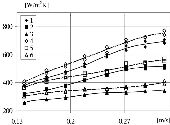
Figure 9. Comparison of heat transfer intensity for the fifth tube in the middle and the side lines of the bundle 1,2,3 – A5 and C5 tubes; 4,5,6 – B5 tube;  $\beta$ : 1, 4 - 0.996; 2, 5 – 0.997; 3, 6 – 0.998.
