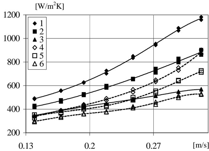
Figure 7. Comparison of heat transfer intensity for the first tube in the middle and the side lines of the bundle 1,2,3 – A1 and C1 tubes; 4,5,6 – B1 tube;  $\beta$ : 1, 4 - 0.996; 2, 5 – 0.997; 3, 6 – 0.998.
