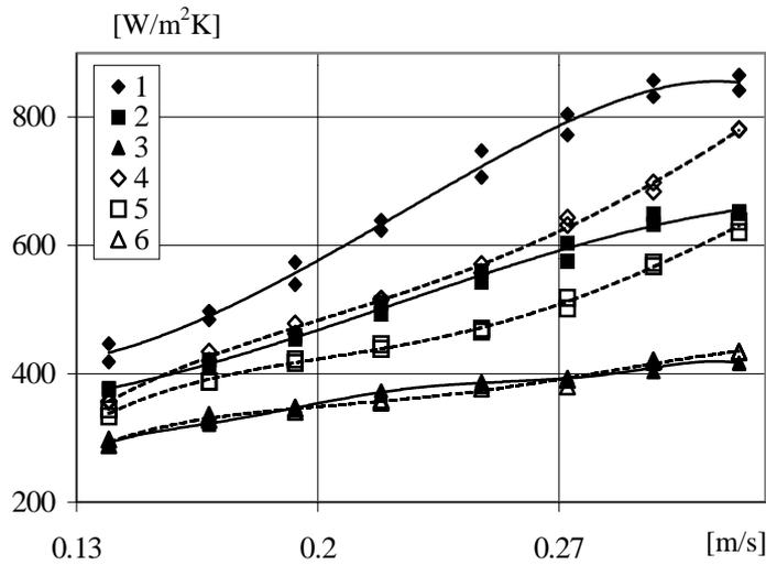
Figure 8. Comparison of heat transfer intensity for the third tube in the middle and the side lines of the bundle 1,2,3 – A3 and C3 tubes; 4,5,6 – B3 tube;  $\beta$ : 1, 4 - 0.996; 2, 5 – 0.997; 3, 6 – 0.998.
