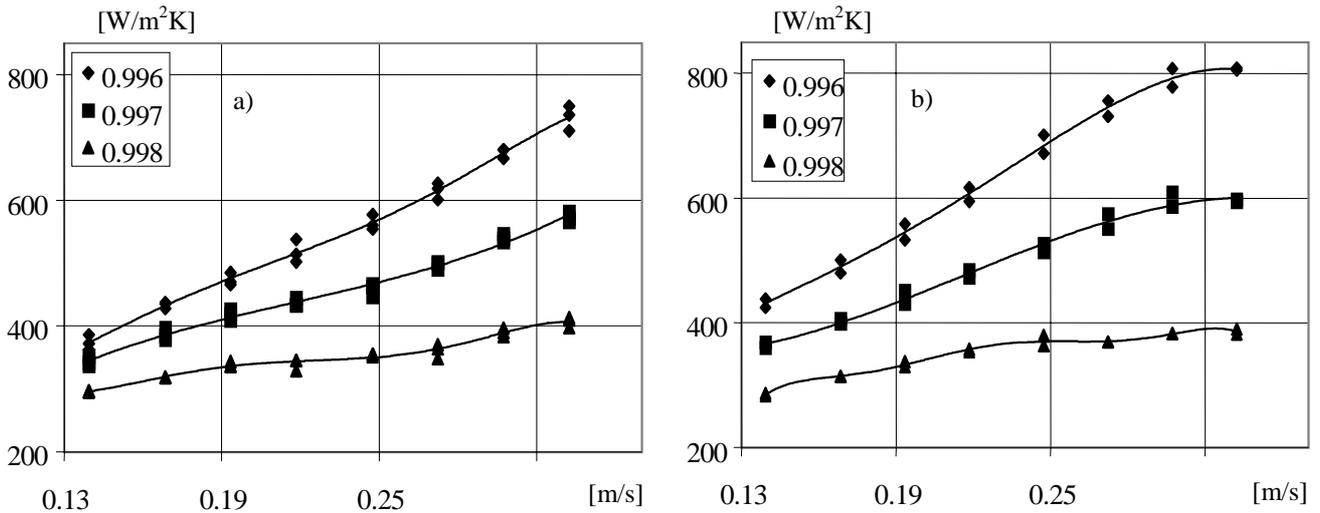
Figure 4. Heat transfer of the tubes of the bundle: a) fourth tube of the middle line (B4); b) fourth tube of the side line (A4 and C4).
