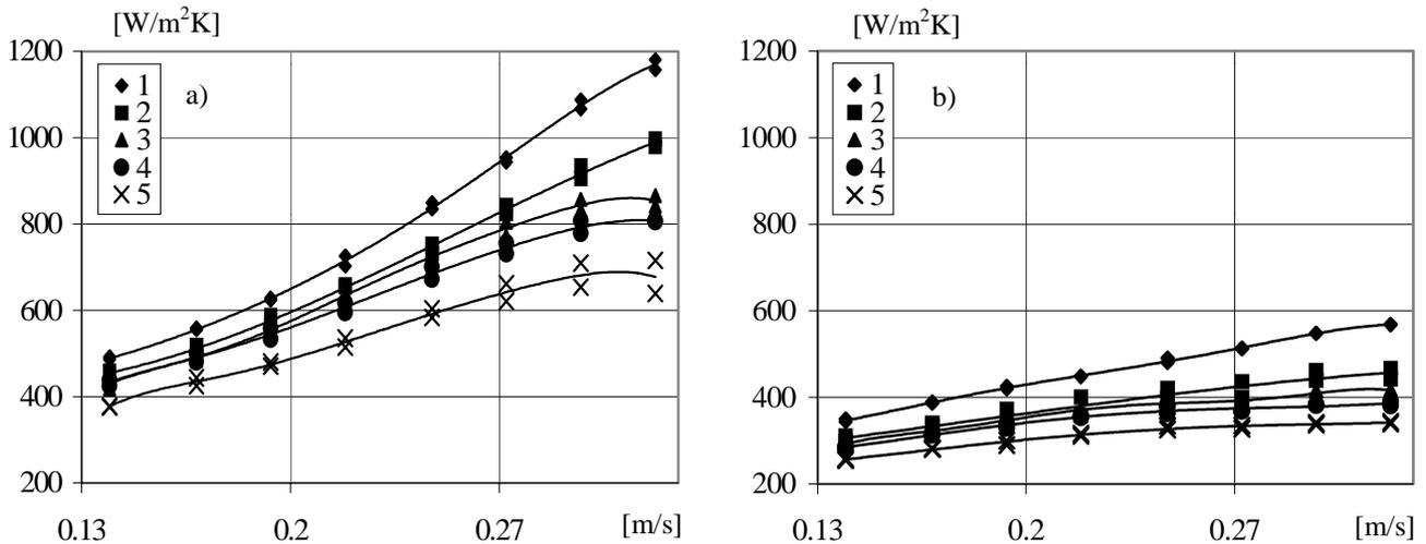
Figure 6. Heat transfer of the side line of the tube bundle: a):  $\beta = 0.996$ ; b):  $\beta = 0.998$ ; 1, 2, 3, 4, 5 – A1, A2, A3, A4, A5 tube correspondingly.
