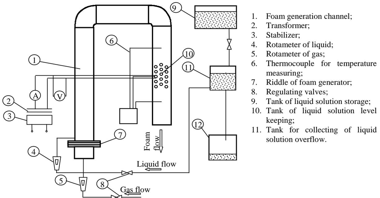
Figure 2. Experimental arrangement.
