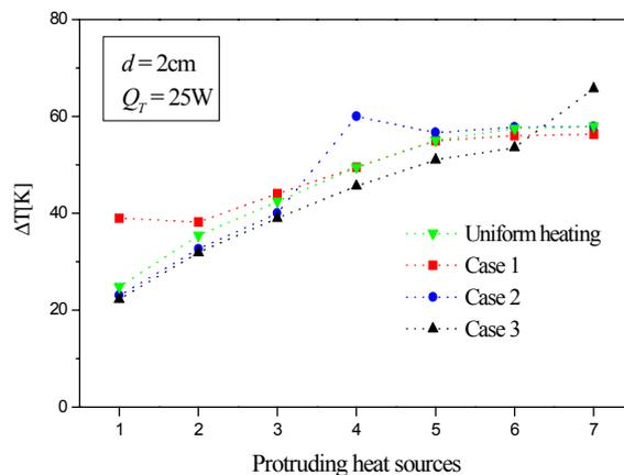
Figure 18 - Temperature excess profiles -  $d = 2cm$  -  $Q_T = 25W$ .
