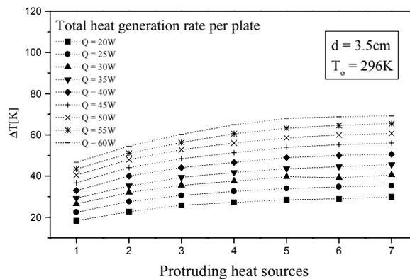
Figure 6 - Temperature excess profiles - Uniform heating -  $d = 3.5\text{cm}$ .
