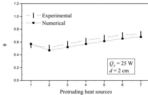
Figure 17 - Numerical and experimental values of temperature excess - non-uniform heating of the plates - case 1.
