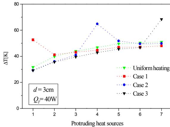
Figure 19 - Temperature excess profiles -  $d = 3\text{cm}$  -  $Q_T = 40\text{W}$ .
