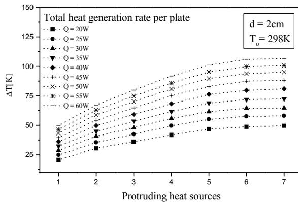
Figure 5 - Temperature excess profiles - Uniform heating -  $d = 2\text{cm}$ .
