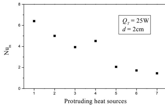
Figure 13 - Averaged Nusselt number in the protruding heat sources - non-uniform heating - case 2 -  $Q_T = 25W$ .
