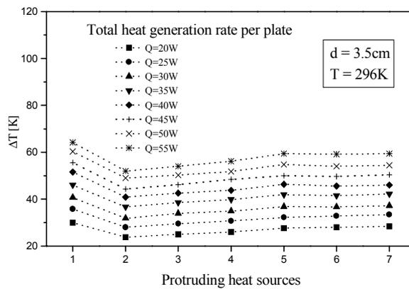
Figure 8 - Temperature excess profiles - Non-uniform heating - case 1 - d = 3.5cm.
