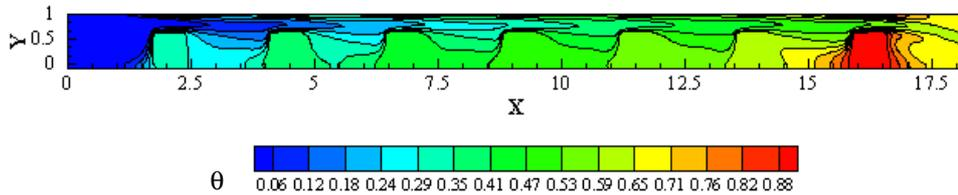
Figure 12 - Isotherms -  $Q_T = 25W$  -  $d = 2.5cm$  - non-uniform heating - case 3 -  $u_o = 0.096$ m/s.
