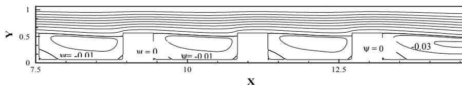
Figure 15 - Streamlines between the forth and the last protrusions -  $Q_T = 25W$  -  $d = 2.5cm$ .
