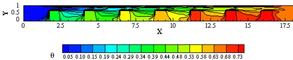
Figure 9 - Isotherms - d = 2cm -  $Q_T = 25W$  – uniform heating -  $u_o = 0.11m/s$ .
