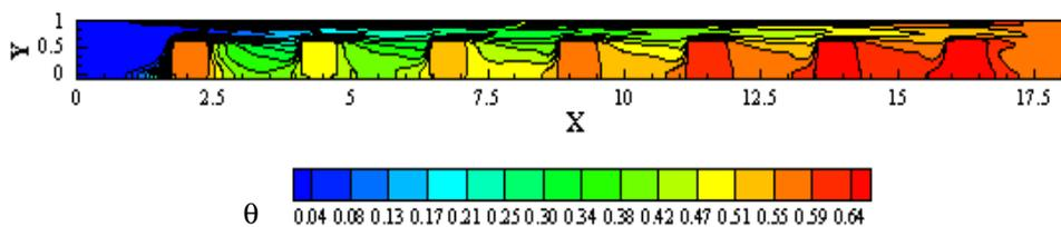
Figure 10 - Isotherms - d = 2cm -  $Q_T = 25W$  – non-uniform heating - case 1 -  $u_o = 0.116m/s$ .
