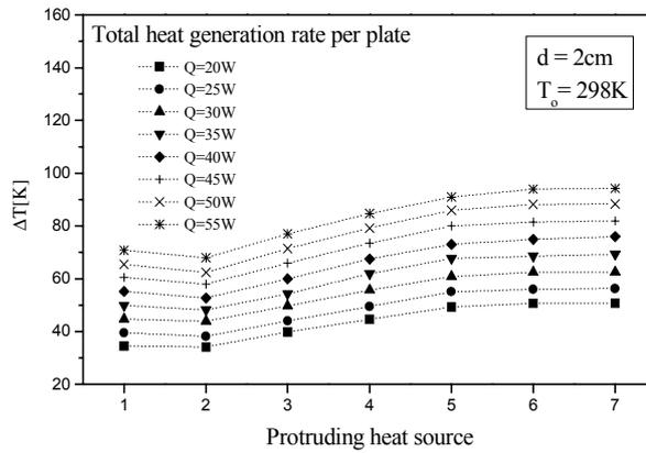
Figure 7 - Temperature excess profiles - Non-uniform heating - case 1 - d = 2cm.
