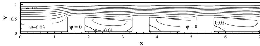
Figure 14 - Streamlines between the channel entrance and the fourth protrusions -  $Q_T = 25W$  -  $d = 2.5cm$ .
