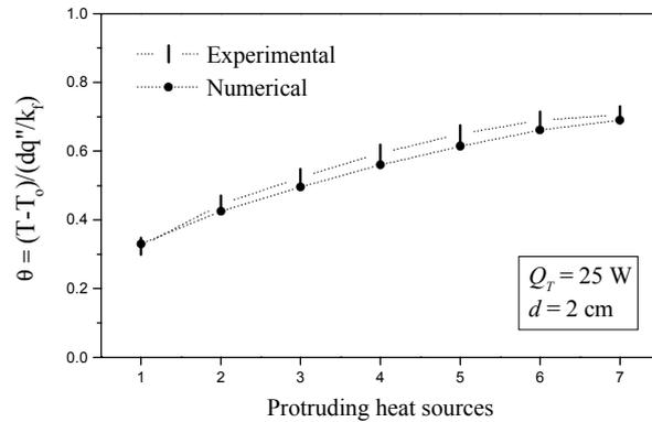
Figure 16 - Numerical and experimental values of temperature excess - uniform heating of the plates.
