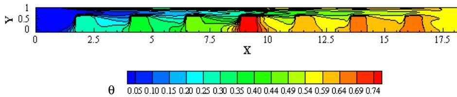
Figure 11 - Isotherms -  $Q_T = 25W$  -  $d = 2cm$  - non-uniform heating - case 2 -  $u_o = 0.10$  m/s.
