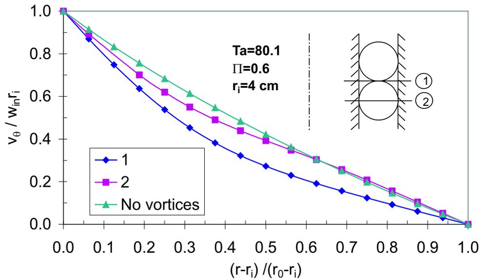
Figure 7: Azimuthal velocity profile before and after the appearance of Taylor vortices.
