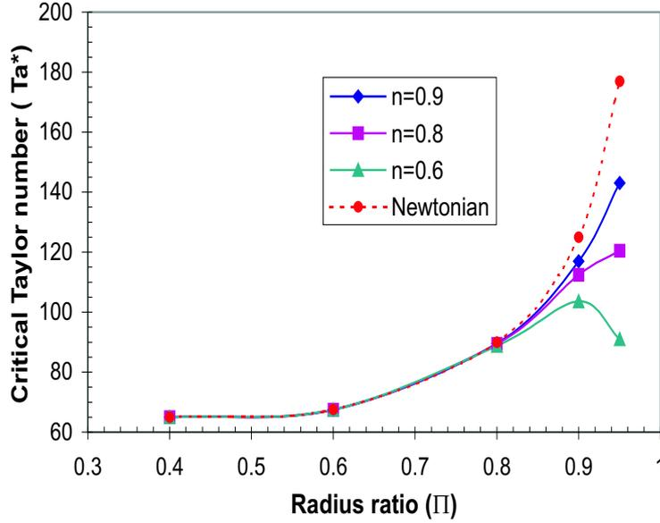
Figure 9: Effect of radii ratio  $\Pi$  on the onset of the instability for viscoplastic liquids.
