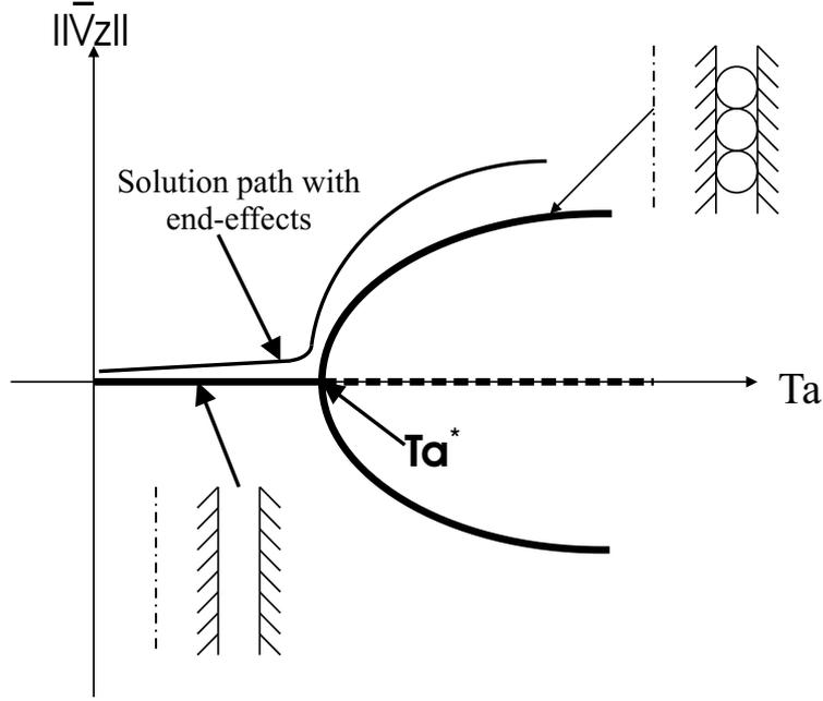
Figure 3: Sketch of the phase diagram of the flow between concentric rotating cylinders. Continuous lines represent stable branches.
