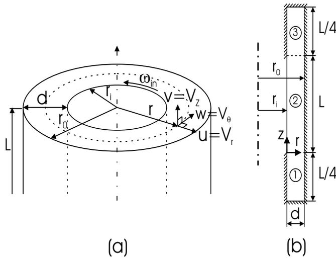
Figure 2: Geometrical configuration of flow between concentric rotating cylinders.
