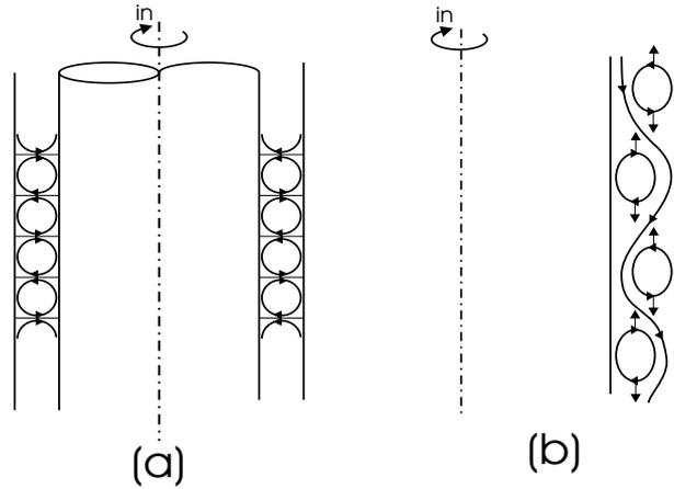
Figure 1: Observed flow patterns: (a) Taylor vortices (b) Helical vortices.
