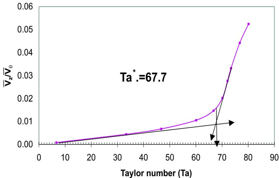
Figure 4: Solution path for Newtonian liquid as Taylor number rises. Radii ratio is  $\Pi = 0.6$ .
