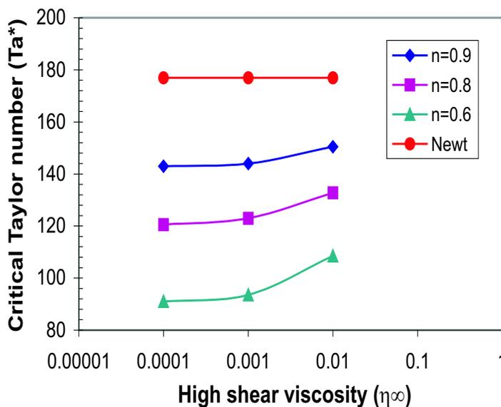
Figure 8: Critical Taylor number as a function of the viscoplastic rheological parameters. Radii ratio is  $\Pi = 0.95$
