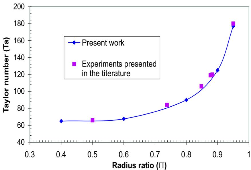
Figure 6: Critical Taylor number for Newtonian liquids as a function of radii ratio  $\Pi \equiv r_i/r_o$
