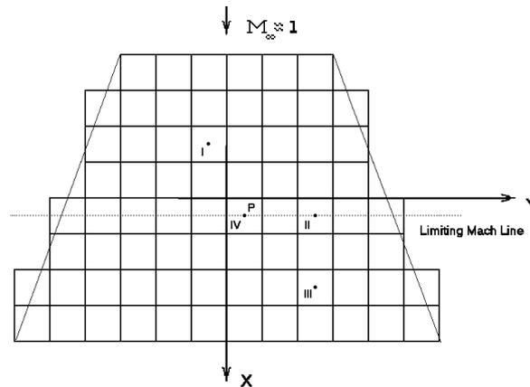
Figure 3. Transformed wing with aspect ratio  $\Lambda = 2.0$  and thickness ratio  $\sigma = 0$  at  $M_\infty = 1.0$ , mapped with  $n_x$  panel along root chord and  $\tilde{n}_y$  panels along its semi-span.
