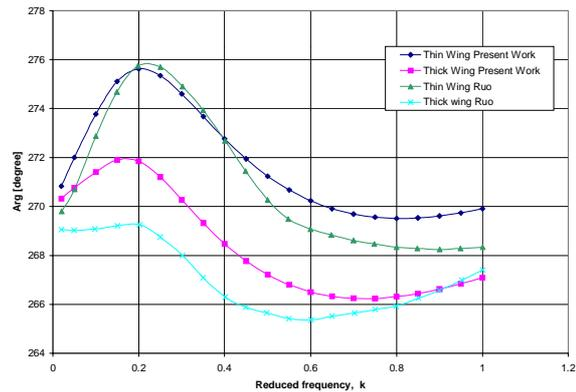
Figure (4.b) argument for an aspect ratio 2.0 rectangular wing in lift due to translation at  $M_\infty = 1.0$ .
