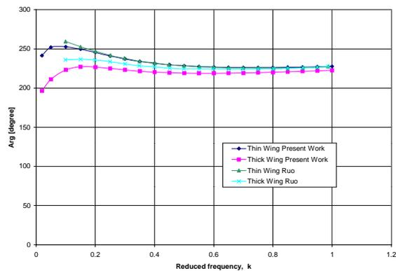
Figure (5.b) argument for an aspect ratio 2.0 rectangular wing in moment due to pitch at  $M_\infty = 1.0$ .
