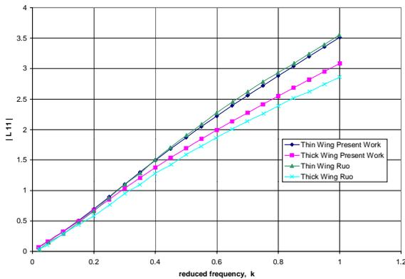
Figure (4.a) amplitude coefficient for an aspect ratio 2.0 rectangular wing in lift due to translation at  $M_\infty = 1.0$ .
