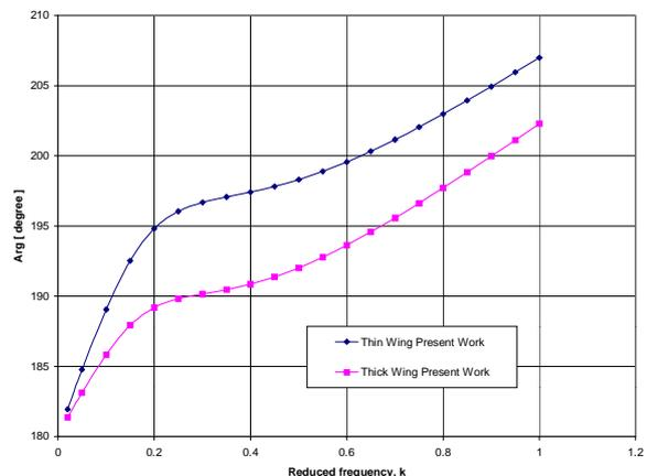
Figure (8.a) amplitude coefficient for an aspect ratio 2.0 rectangular wing in lift due to pitch at  $M_\infty = 1.0$ .
