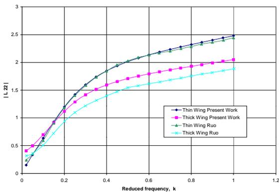
Figure (5.a) amplitude coefficient for the moment due to pitch for an aspect ratio 2.0 rectangular wing at  $M_\infty = 1.0$ .
