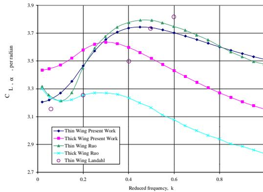
Figure 6. Lift-slope curve variation with reduced frequency and thickness for  $\Lambda= 2.0$  rectangular wing at  $M_\infty = 1.0$ .
