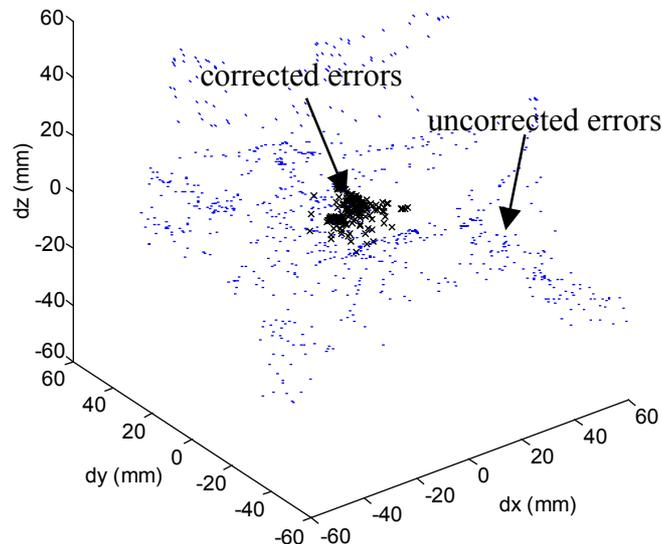
Figure 5. Measured and Residual Errors After Compensation
