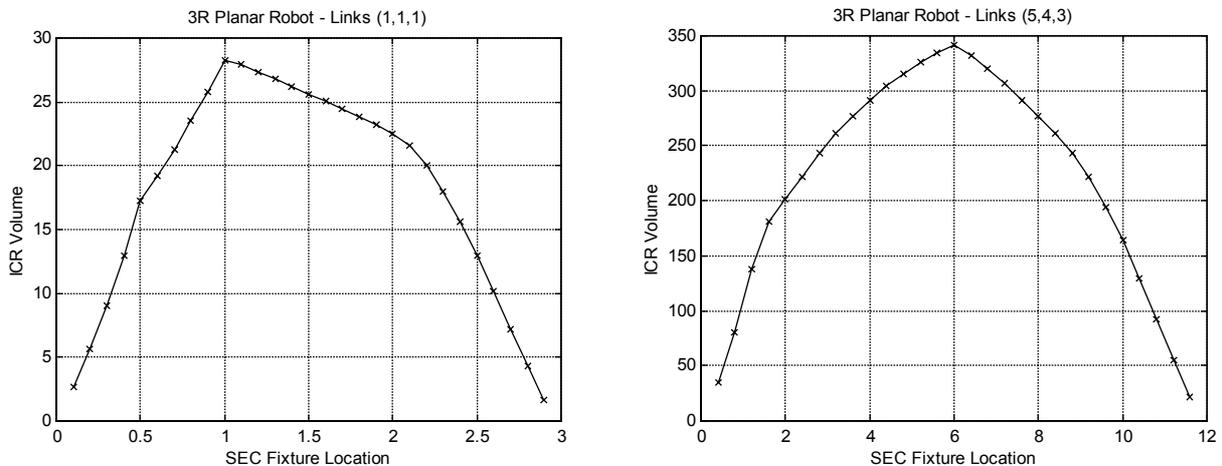
Figure 2. ICR Volume as a Function of the Fixture Location for Link Lengths  $(1, 1, 1)$  and  $(5, 4, 3)$
