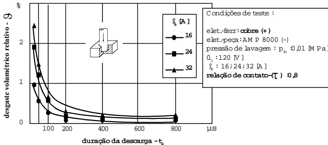
Figure 8. Volumetric relative wear  $\vartheta$  for duty factor  $\tau$  of 0,8.
