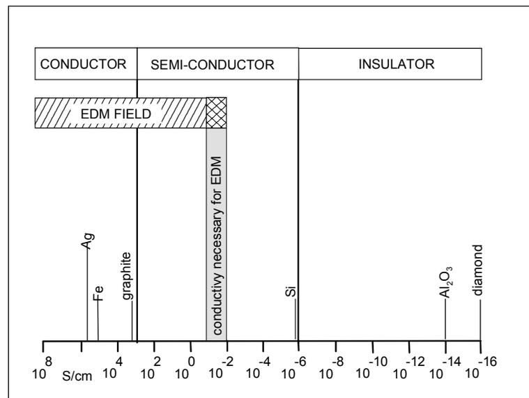
Figure 1. Electrical Conductivity necessary for EDM (König, Klocke & Lenzen, 1996)
