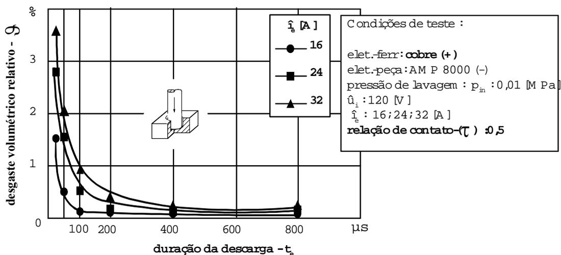
Figure 7. Volumetric relative wear  $\vartheta$  for duty factor  $\tau$  of 0,5.
