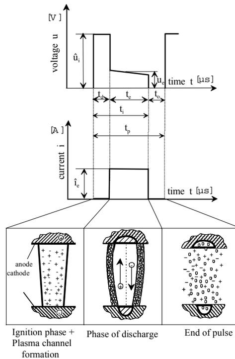
Figure 2. The phases of an electric discharge in EDM (König and Klocke, 1997)
