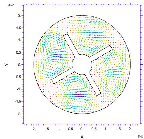
Figure 4b. Secondary flow in the curved annular duct cross-section at Dean number = 70 and angle =  $30^\circ$
