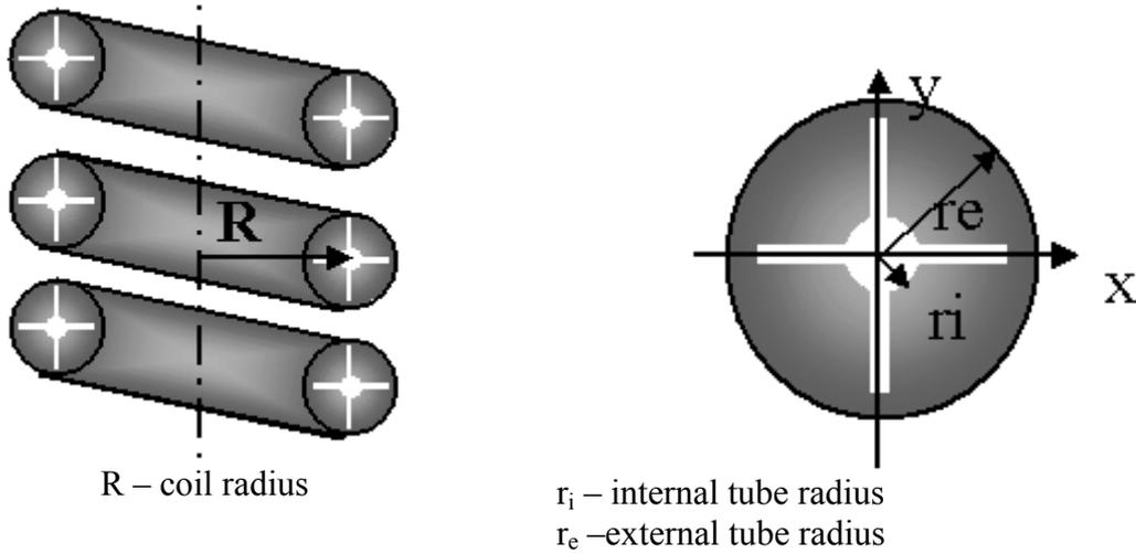
**Figure 1.** Schematic representation of the curved annular duct with four rectangular fins.
