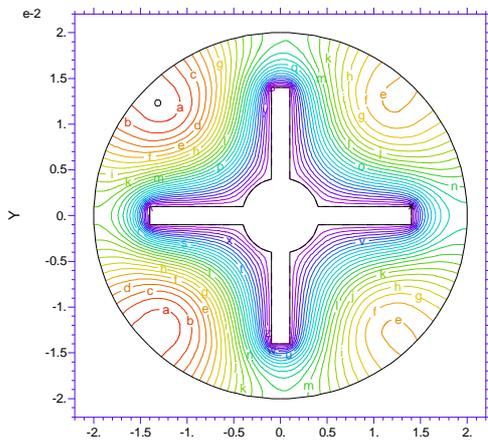
Figure 5a. Temperature field at Dean number = 0.9 and angle =  $0^\circ$
