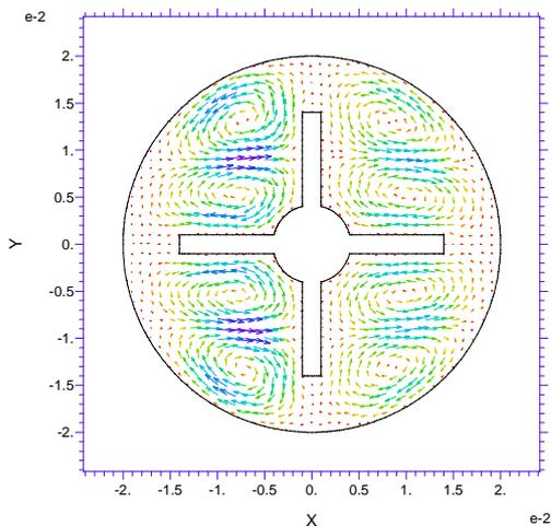
Figure 4a. Secondary flow in the curved annular duct cross-section at Dean number = 70 and angle =  $0^\circ$
