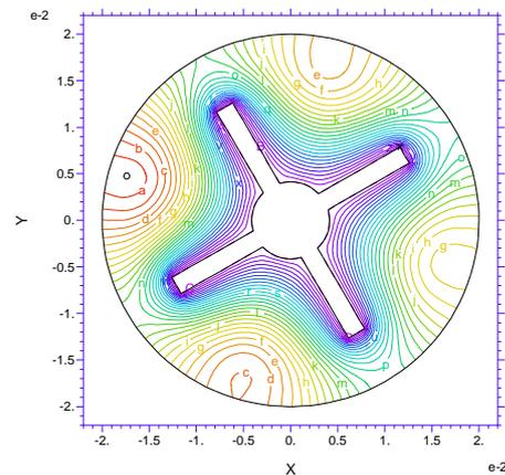
Figure 5b. Temperature field at Dean number = 0.9 and angle =  $30^\circ$
