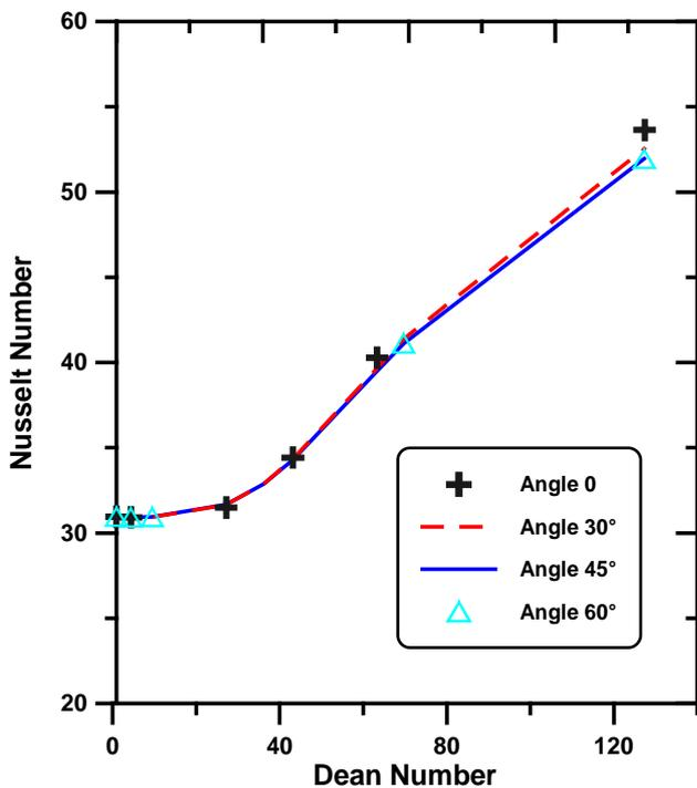
Figure 6 Nusselt number results for concentric curve circular ducts with four rectangular fins.
