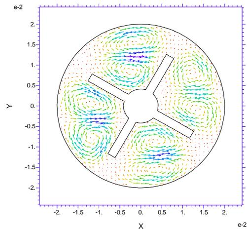
Figure 4d. Secondary flow in the curved annular duct cross-section at Dean number = 70 and angle =  $60^\circ$
