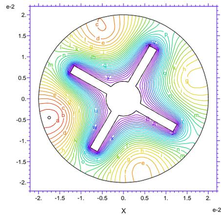
Figure 5c. Temperature field at Dean number = 0.9 and angle = 45°
