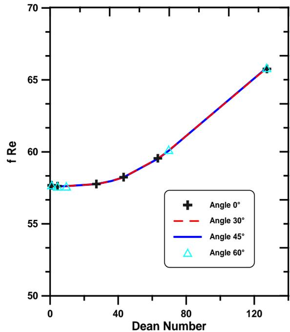
Figure 7. Friction factor results for the concentric curve circular ducts with four rectangular fins.
