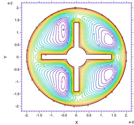
Figure 3. The average velocity ( $w/w_m$ ) for Dean number = 127 and fin angle = 0.
