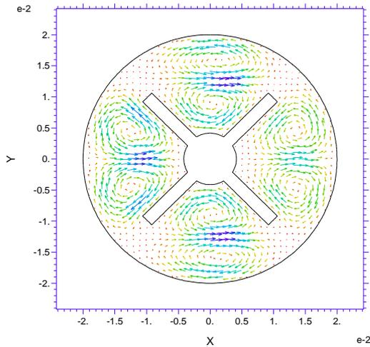
Figure 4c. Secondary flow in the curved annular duct cross-section at Dean number = 70 and angle =  $45^\circ$
