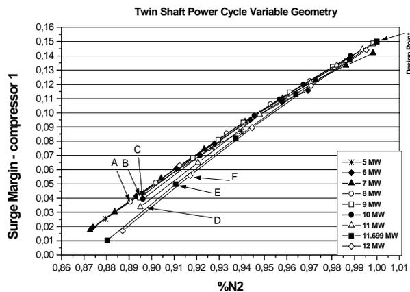
Figure 14. Surge margin versus corrected speed
