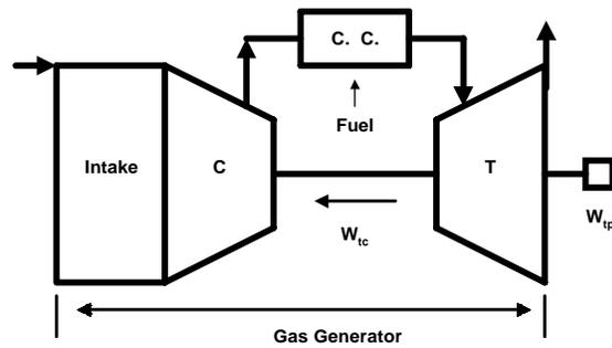
Figure 2. Single shaft power generator
