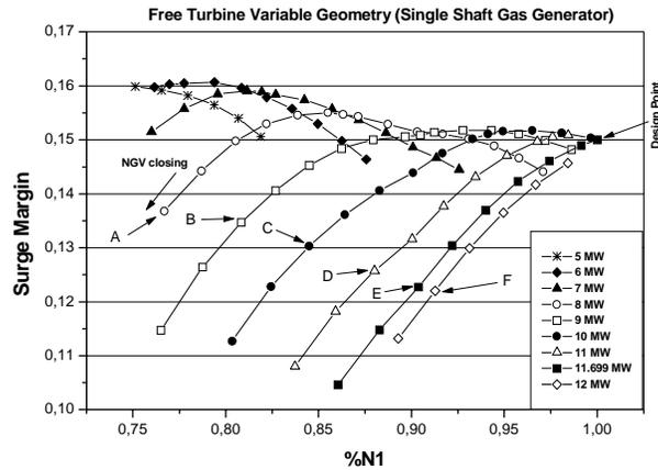
Figure 12. Surge margin versus corrected speed
