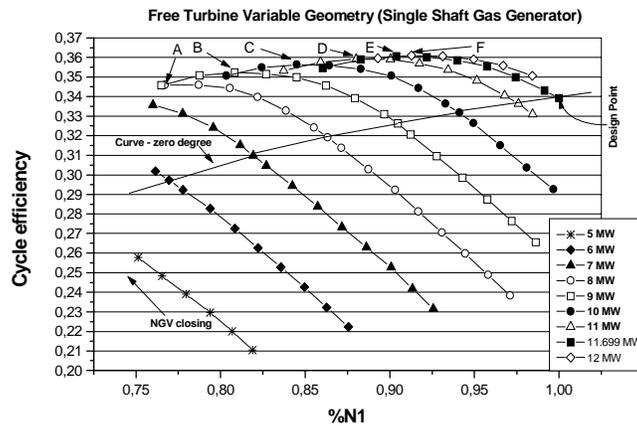
Figure 5. Cycle efficiency versus corrected speed
