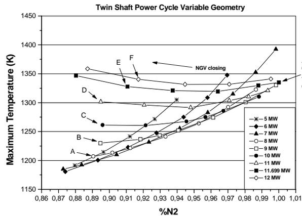
Figure 10. Maximum cycle temperature versus corrected speed
