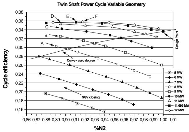
Figure 7. Cycle efficiency versus corrected speed
