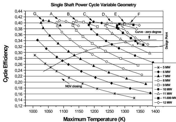
Figure 6. Cycle efficiency versus maximum cycle temperature
