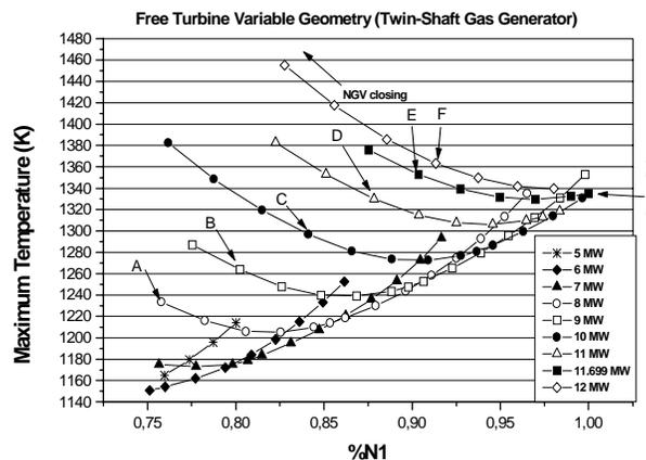
Figure 11. Maximum cycle temperature versus corrected speed
