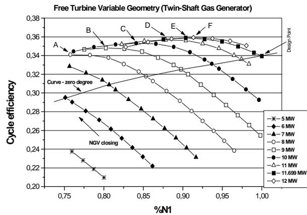
Figure 8. Cycle efficiency versus corrected speed
