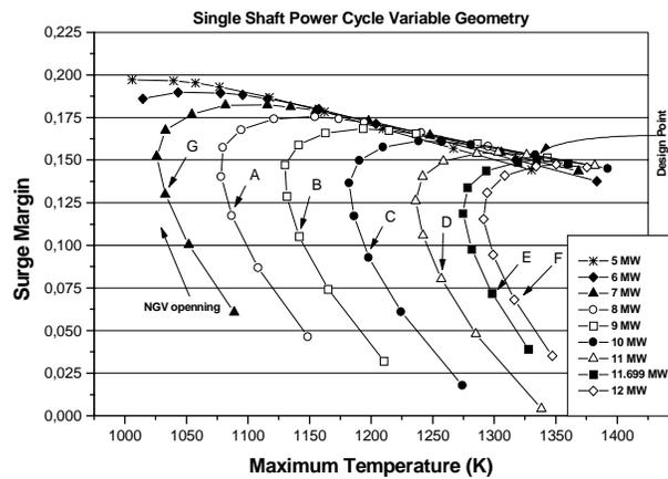
Figure 13. Surge margin versus maximum cycle temperature
