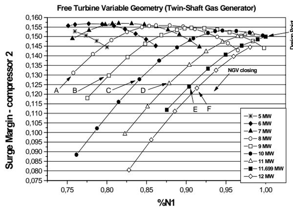
Figure 17. Surge margin versus corrected speed
