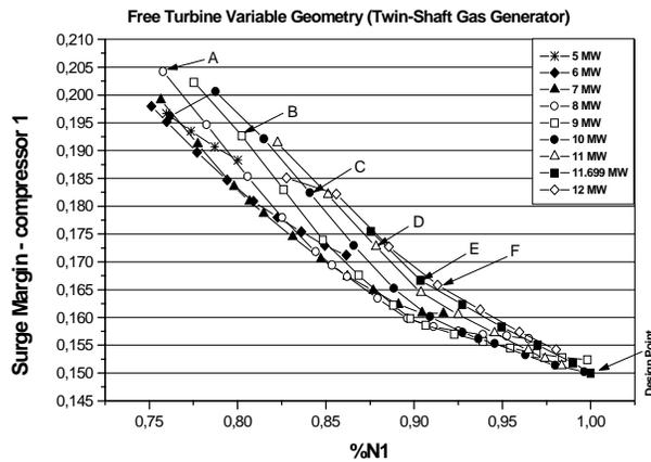
Figure 16. Surge margin versus corrected speed
