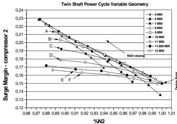
Figure 15. Surge margin versus corrected speed
