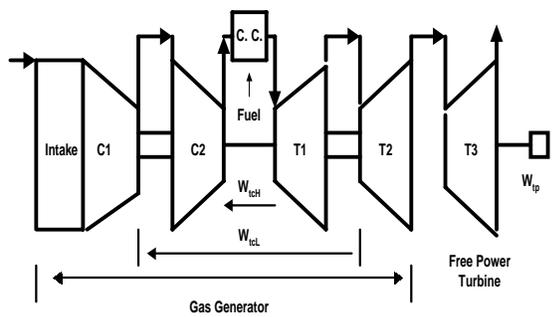
Figure 4. Free turbine (twin shaft gas generator)
