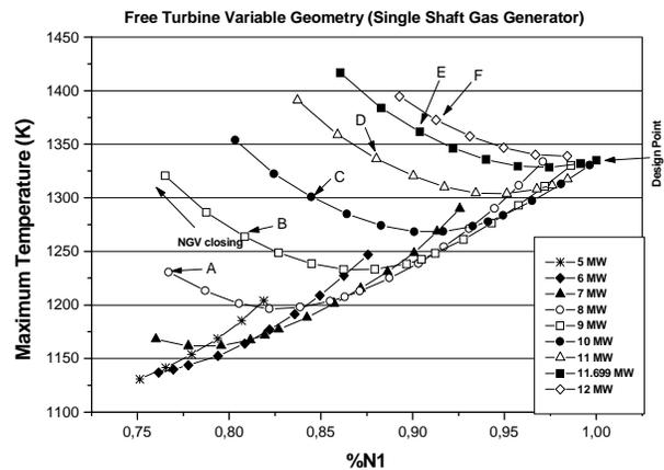
Figure 9. Maximum cycle temperature versus corrected speed
