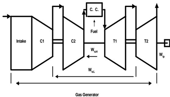
Figure 3. Twin shaft power generator
