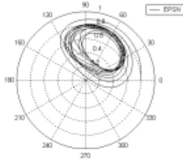
Figure 6. Case IV:  $\varepsilon = 0.8$ ,  $W = 33.6$  Kg,  $c = 2.54e-4$  m,  $r_b = 2.54e-2$  m,  $L = 5.08e-2$  m,  $F_u = 100$  N,  $V_b = 5000$  rpm,  $\eta = 8.276e-3$   $Ns/m^2$ .
