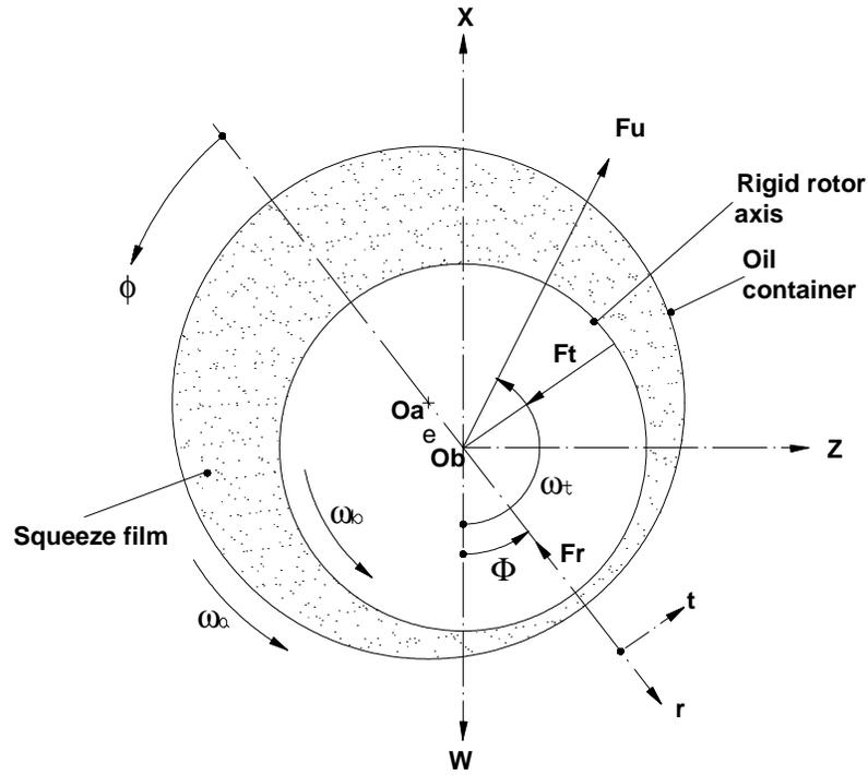
Figure 1. Squeeze film damper with the dynamic forces and coordinates defined.
