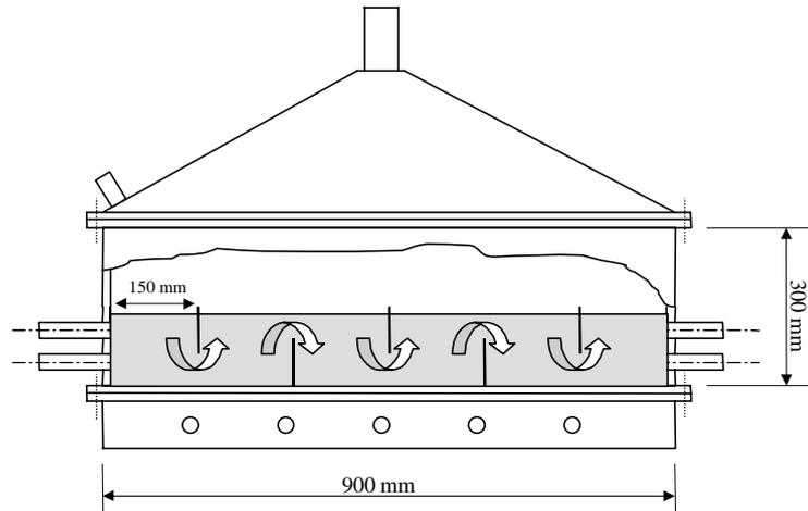
**Figure 3** – View of the heat exchanger with baffles
