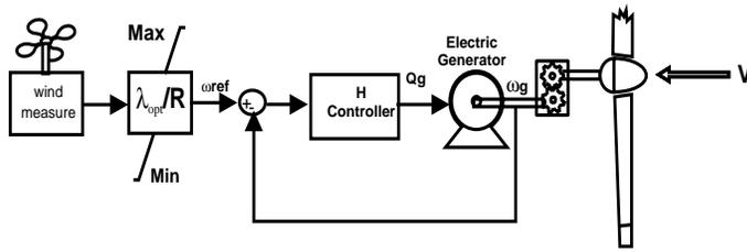
Figure 4: Control block diagram
