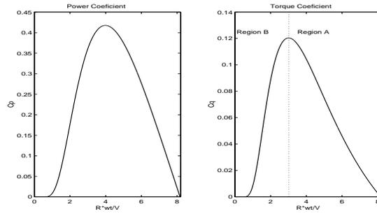
Figure 2:  $C_p(\lambda)$  and  $C_q(\lambda)$  of MOD-2 wind turbine
