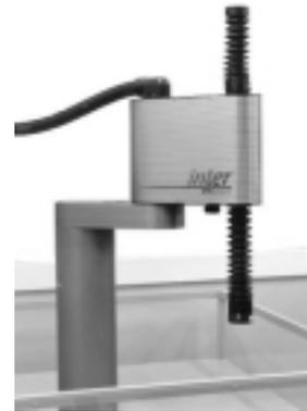
**Figura 1. Robô SCARA**
