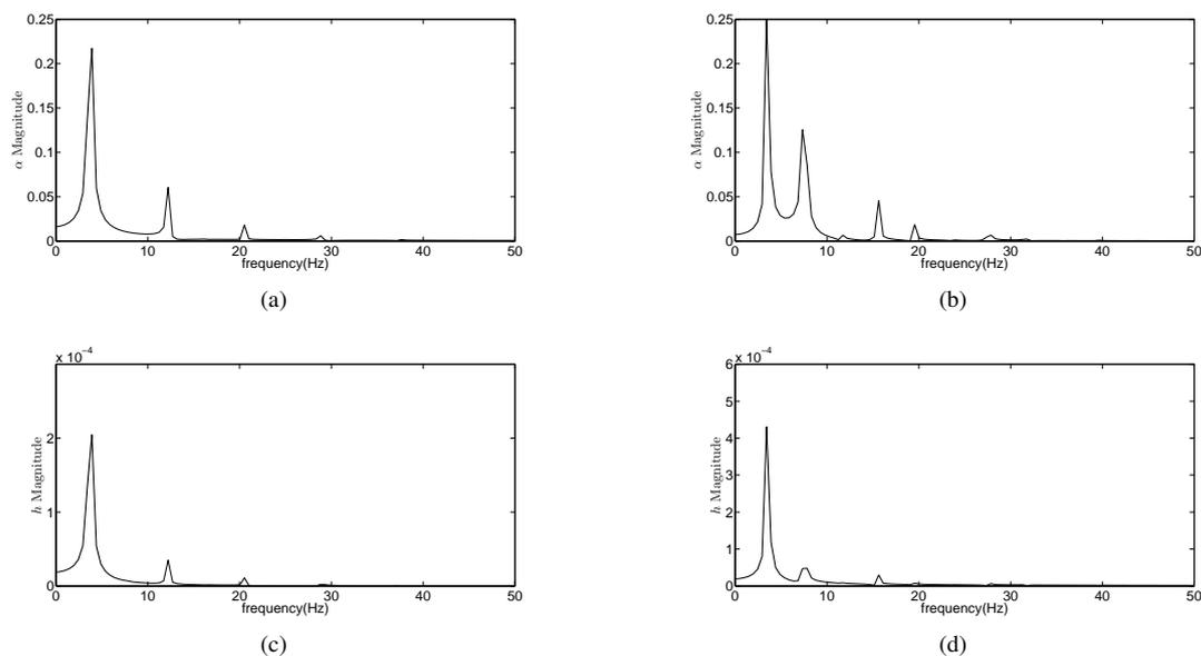
**Figure 12:** Power spectrum of the pitch and plunge motions (a,c) before the first transition ( $13.3m/s$ ) and (b,d) after the first transition ( $13.5m/s$ ).
