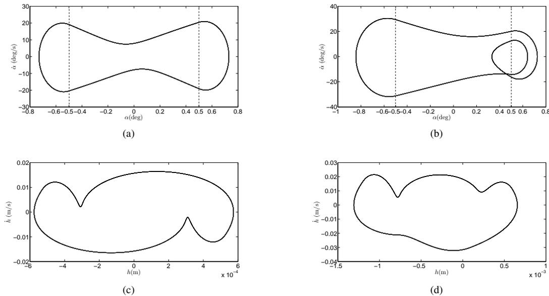
**Figure 13:** Phase portrait of the pitch and plunge motions (a,c) before the first transition ( $13.3m/s$ ) and (b,d) after the first transition ( $13.5m/s$ ).
