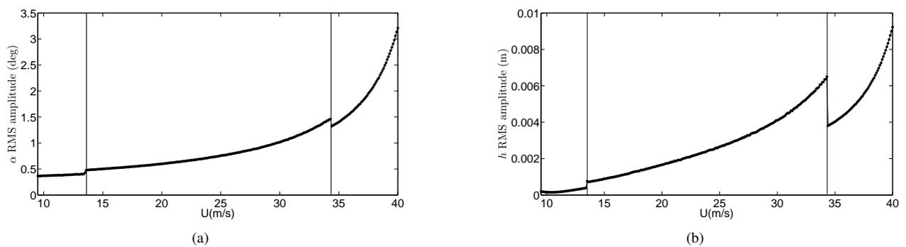
Figure 10: Variations of (a) RMS pitch amplitude and (b) RMS plunge amplitude when increasing the freestream velocity.
