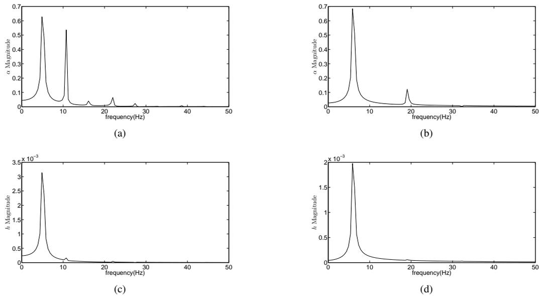
**Figure 15:** Power spectra of the pitch and plunge motions (a,c) before the second transition ( $34, 2m/s$ ) and (b,d) after the second transition ( $34, 4m/s$ ).
