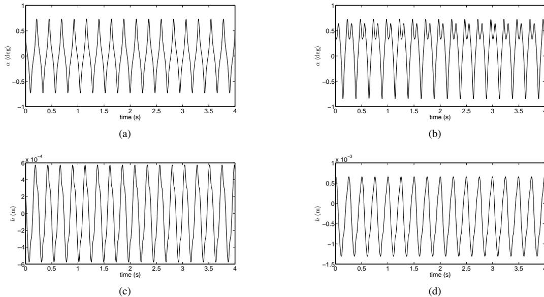
**Figure 11:** Time histories of the pitch and plunge motions (a,c) before the first transition ( $13.3m/s$ ) and (b,d) after the first transition ( $13.5m/s$ ).
