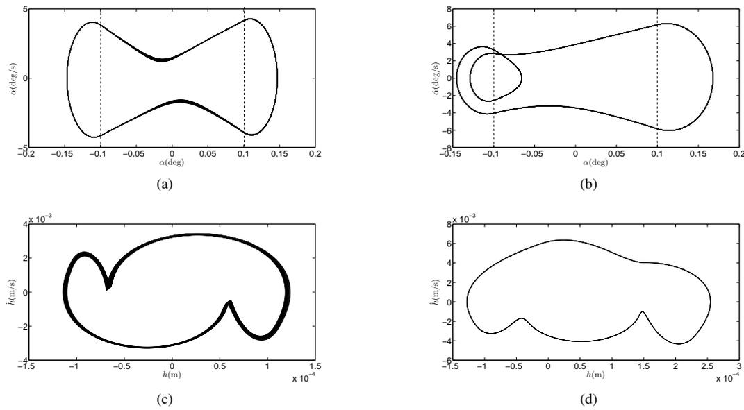
**Figure 6:** Phase portrait of the pitch and plunge motions (a,c) before the first transition ( $13.3m/s$ ) and (b,d) after the first transition ( $13.5m/s$ ).
