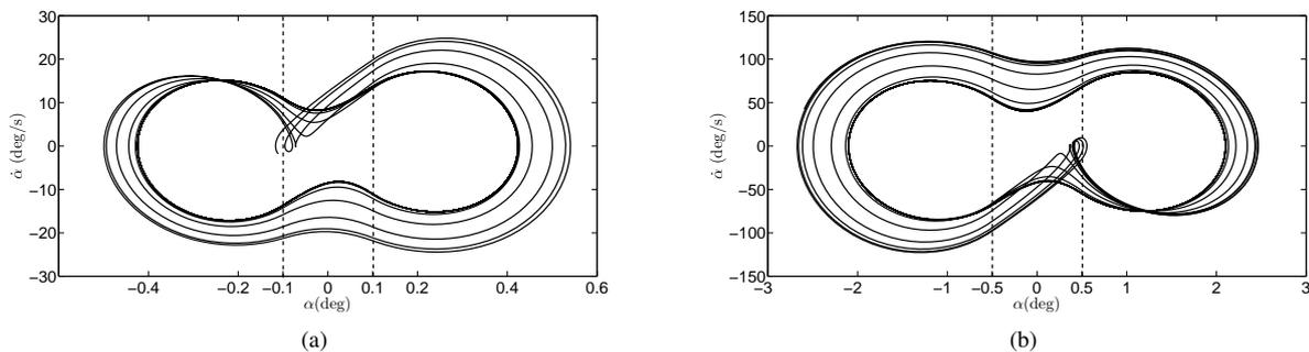
**Figure 17:** Phase portrait at transition speed for pitch motion: (a) freeplay of 0.1 degrees (34.4 m/s), (b) freeplay of 0.5 degrees (34.3 m/s)
