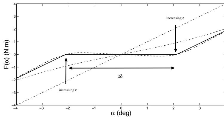
**Figure 2:** Pitch angle versus torque described in Eq. (3),  $\varepsilon$  increasing from 0 to 100
