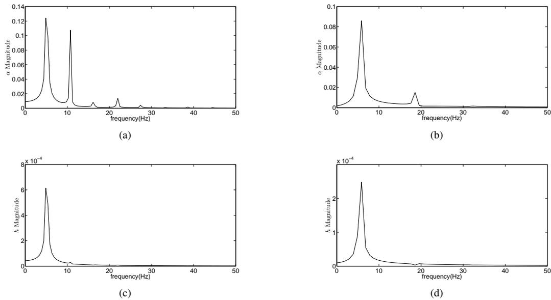
Figure 8: Power spectra of the pitch and plunge motions (a,c) before the second transition ( $34.3m/s$ ) and (b,d) after the second transition ( $34.5m/s$ ).
