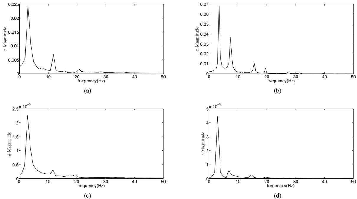
**Figure 5:** Power spectra of the pitch and plunge motions (a,c) before the first transition ( $13.3m/s$ ) and (b,d) after the first transition ( $13.5m/s$ ).
