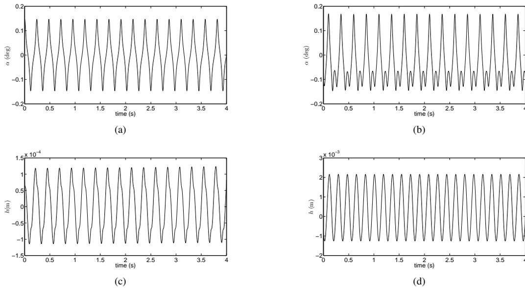
**Figure 4:** Time series of the pitch and plunge motions (a,c) before the first transition ( $13.3m/s$ ) and (b,d) after the first transition ( $13.5m/s$ ).
