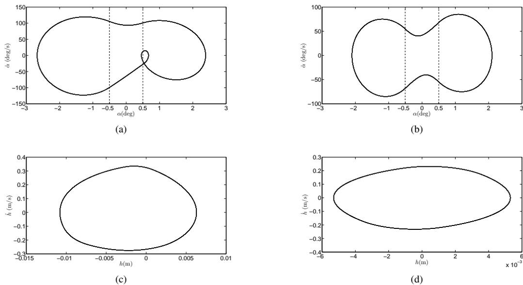
**Figure 16:** Phase portrait of the pitch and plunge motions (a,c) before the second transition ( $34, 2m/s$ ) and (b,d) after the second transition ( $34, 4m/s$ ).
