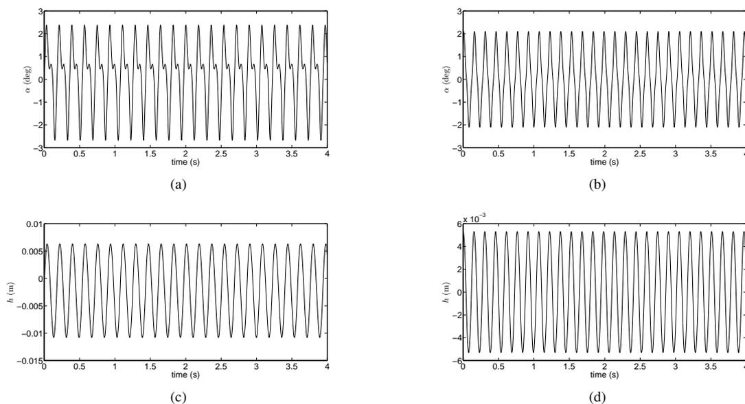
**Figure 14:** Time histories of the pitch and plunge motions (a,c) before the second transition ( $34, 2m/s$ ) and (b,d) after the second transition ( $34, 4m/s$ ).
