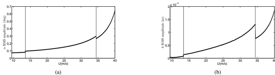
**Figure 3:** Variations of (a) RMS pitch amplitude and (b) RMS plunge amplitude when increasing the freestream velocity.
