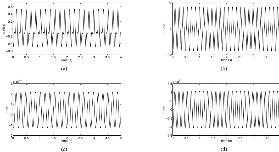
**Figure 7:** Time histories of the pitch and plunge motions (a,c) before the second transition ( $34.3m/s$ ) and (b,d) after the second transition ( $34.5m/s$ ).
