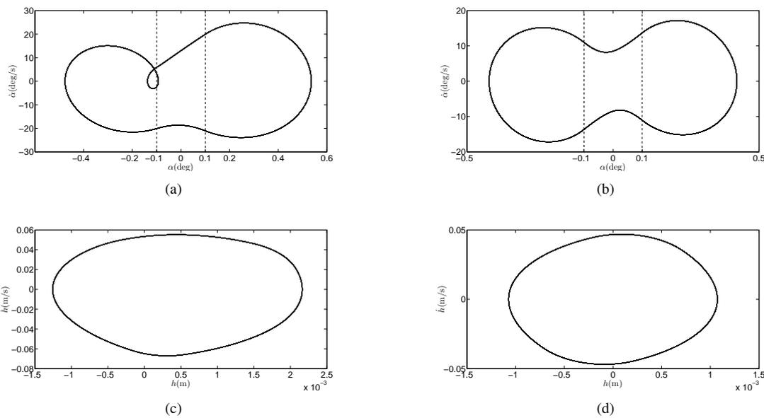
Figure 9: Phase portrait of the pitch and plunge motions (a,c) before the second transition ( $34.3m/s$ ) and (b,d) after the second transition ( $34.5m/s$ ).
