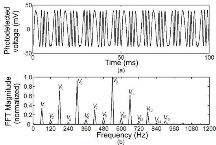
Figure 4. Typical output interferometric signal observed when the MAPFA is driven with a sinusoidal voltage.
