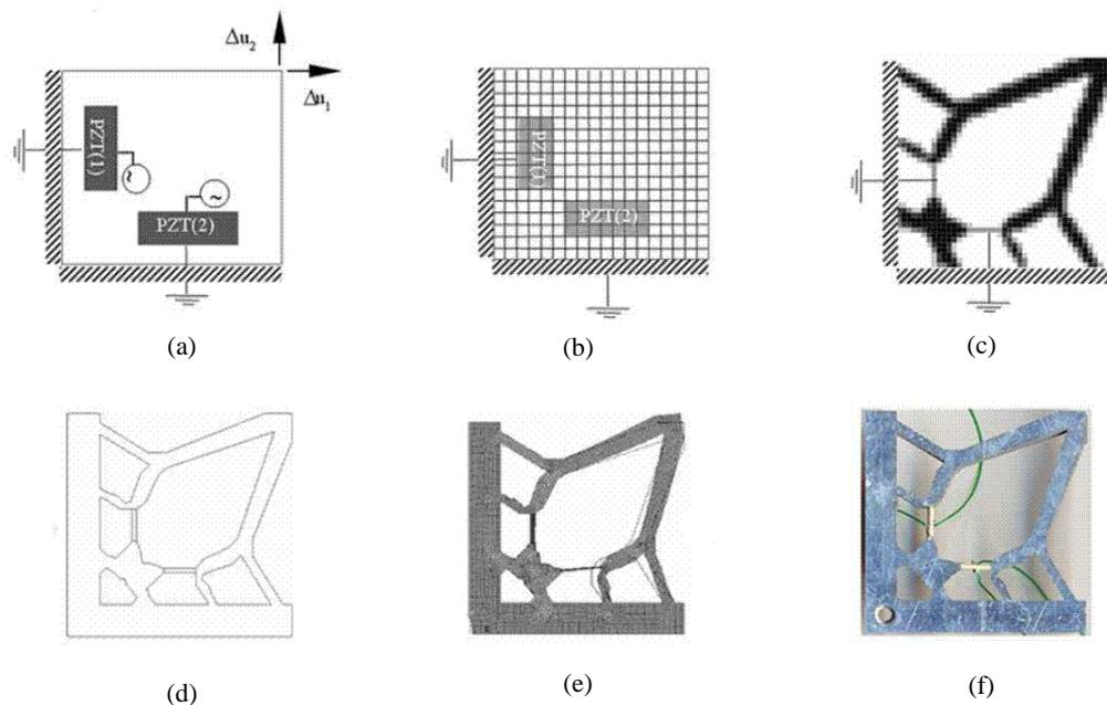
Figure 1. Topology optimization procedure for designing piezoelectric mechanisms ( $\Delta u$  is the desired output displacement) (Carbonari et al, 2009). a) Initial domain, b) Domain discretized, c) Topology obtained, d) Interpretation, e) Verification, and f) Manufactured.
