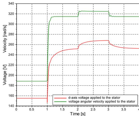
Figure 22. SSMPC load response:  $v_{ds}$  and  $\omega_e$ .
