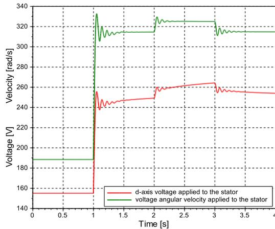
Figure 16. DMC load response:  $v_{ds}$  and  $\omega_e$ .
