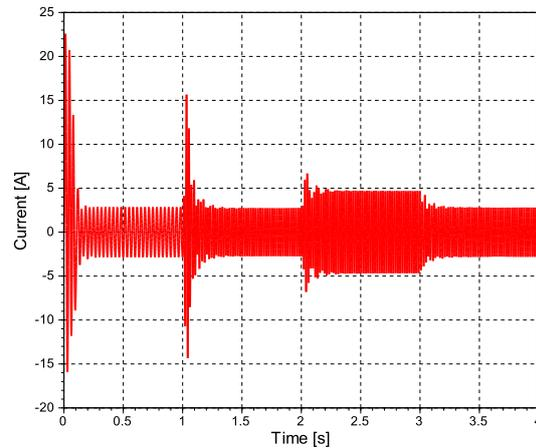
Figure 17. DMC load response:  $i_{as}$ .
