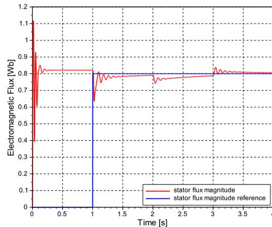
Figure 15. DMC load response:  $|\lambda_s|$ .
