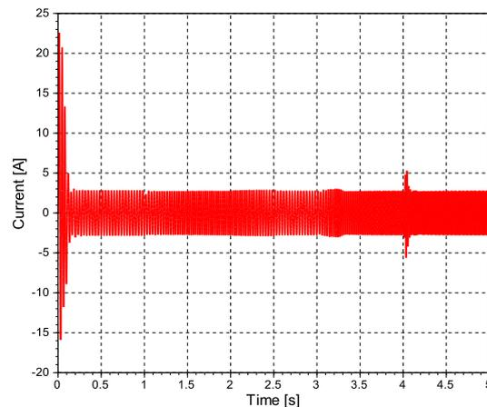
Figure 19. SSMPC response: stator A-phase current  $i_{as}$ .
