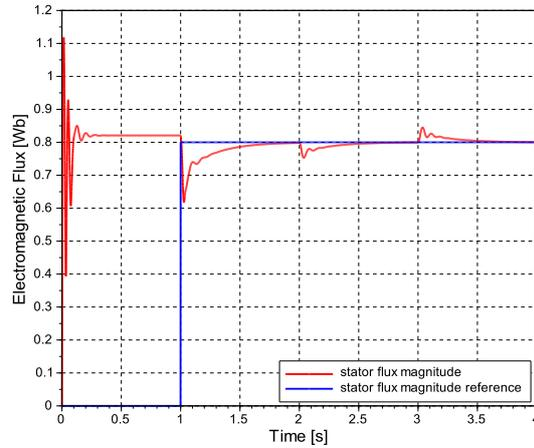
Figure 21. SSMPC load response:  $|\lambda_s|$ .
