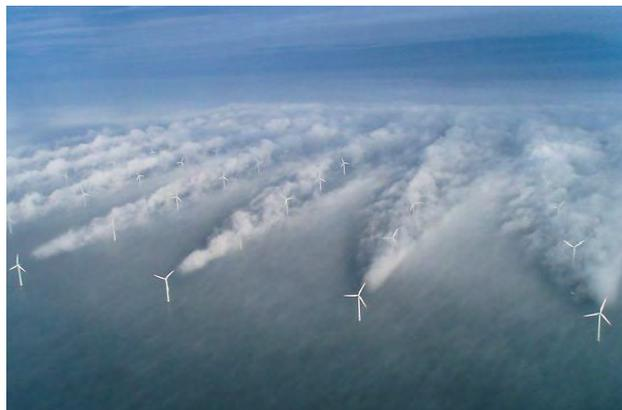
Figure 1. Aerial image of the effects of wake at a wind farm offshore in Denmark, ([www.ecn.nl](http://www.ecn.nl))
