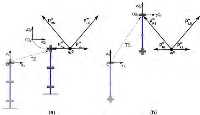
Figure 4: Frame reference transformation: (a) transformation to the right leg; (b) transformation to the right arm.
