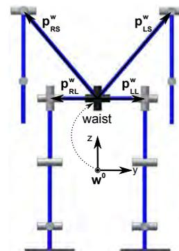
Figure 2: 3D Model of an humanoid structure.
