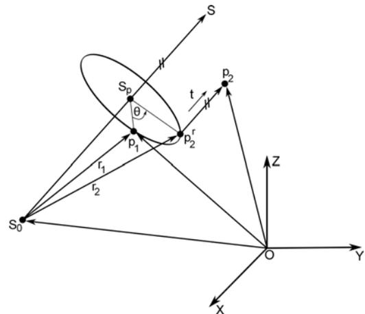
Figure 1: Vector diagram of a spatial displacement.
