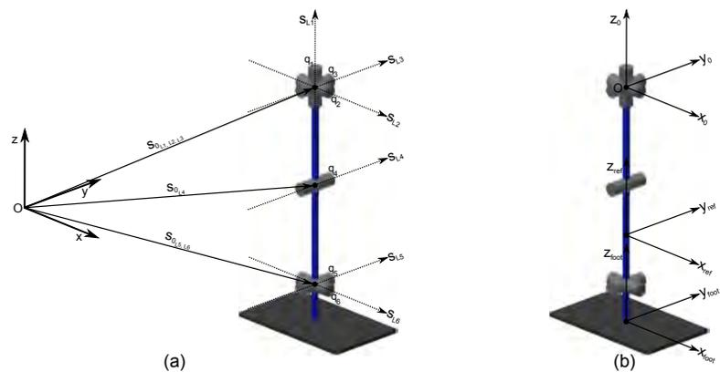
Figure 3: Kinematic chain that represents one leg: (a) identification of the screw parameters; (b) three reference frames allocated in the leg.
