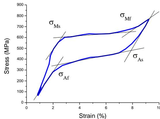
**Figure3.** Schema showing the tangent method used to define the phase transformation stresses in a stress vs. strain loop.
