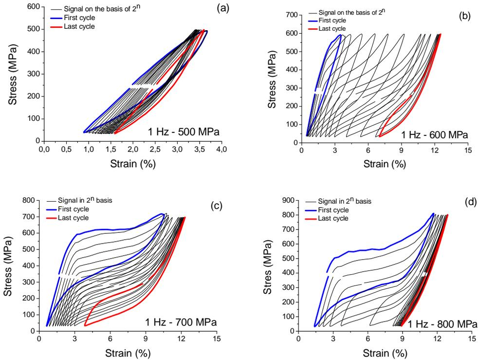
**Figure 5.** Evolution of the superelastic behavior of the studied NiTi SMA wire at 1 Hz under 500, 600, 700 and 800 MPa.
