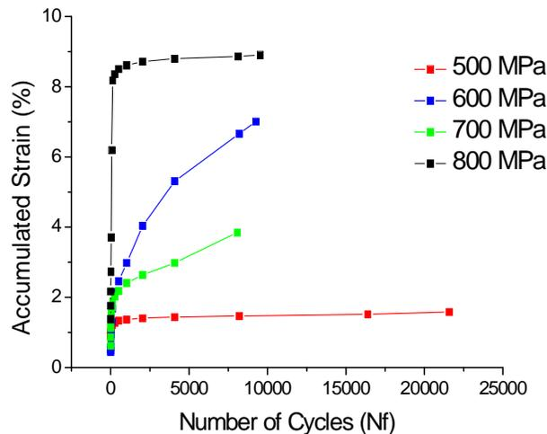
**Figure 7.** Accumulated permanent strain in the NiTi SMA wire during cycling under 500, 600, 700 and 800 MPa at 1Hz.
