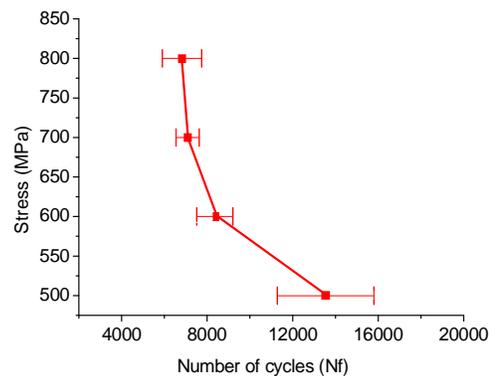
**Figure 10.** Wohler curve for each stress level applied in the studied NiTi SMA wire at 1 Hz.
