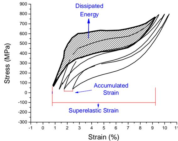
**Figure 2.** Schematic representation of the superelastic behavior for  $n$  fatigue cycles until failure.
