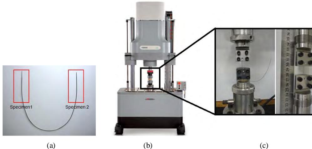
**Figure 1.** NiTi SMA superelastic wire and testing machine. (a) NiTi superelastic orthodontic wire with 0.50 mm in diameter. (b) Electrodynamic testing machine (Instron E10000). (c) Detail of the NiTi arch wire assembled for testing.
