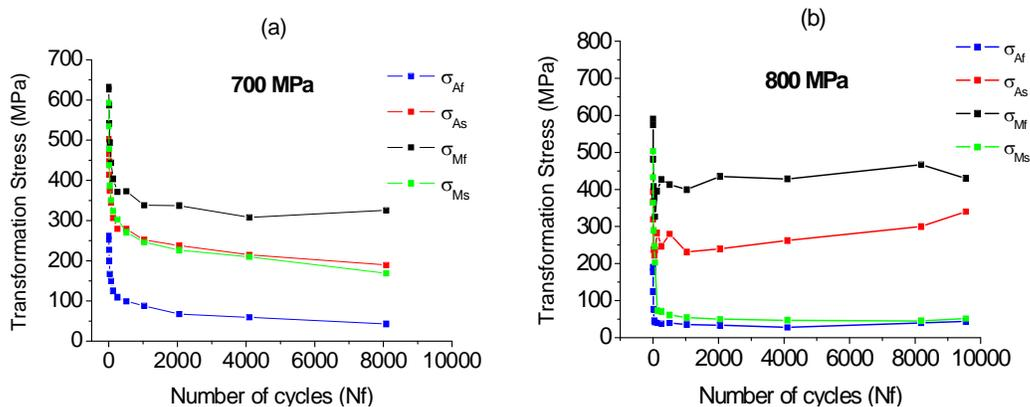
**Figure 9.** Evolution of the critical stresses during phase transformation of NiTi SMA wires. (a) For superelastic stress amplitude of 700 MPa. (b) For superelastic stress amplitude of 800 MPa.
