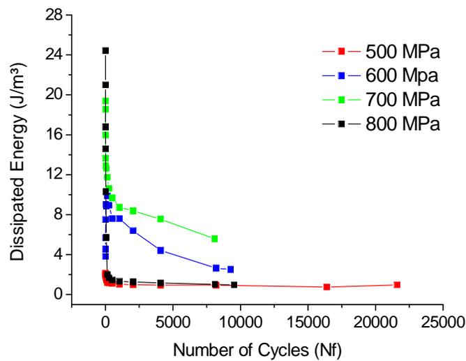
**Figure 6.** Dissipated energy by the NiTi SMA wire at 1Hz under 500, 600, 700 and 800 MPa.
