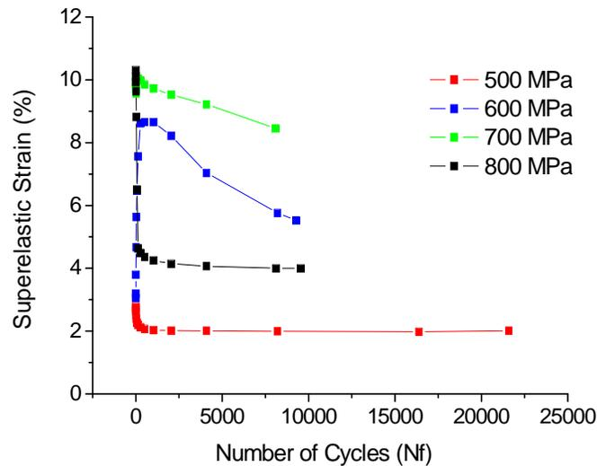
**Figure 8.** Reversible superelastic strain in the NiTi SMA wire for 500, 600, 700 and 800 MPa at 1Hz.
