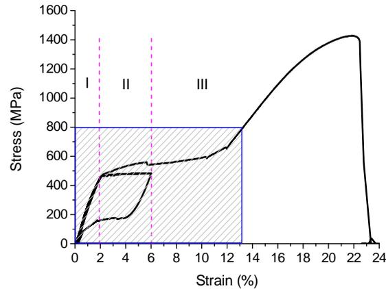
**Figure 4.** Stress vs. strain behavior for the monotonic tensile test in NiTi SMA wire used to study the functional fatigue.
