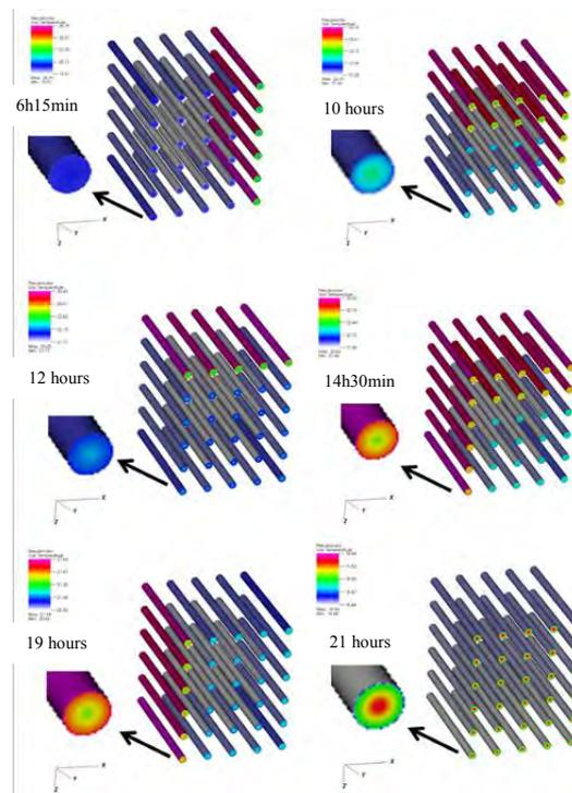
Figure 5. Results for 3D application Visit (2008), the tube wall temperature and fluid (inside tubes) to 6h15min, 10 hours, 12 hours, 14h30min, 19 hours and 21 hours on the first day of computer simulation.
