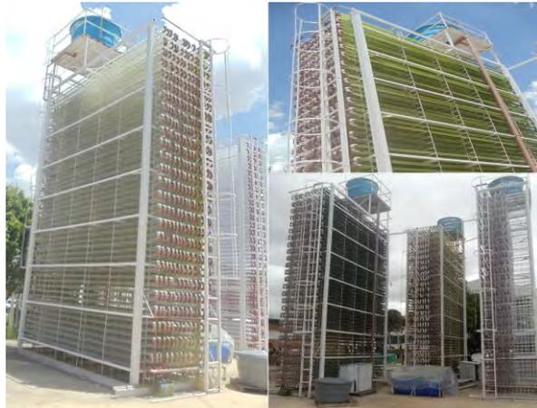
Figure 1. Compact tubular photobioreactor (CTP) NPDEAS.
