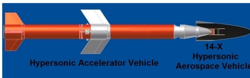
Figure 4: Hypersonic Accelerator Vehicle and VHA 14-X.
