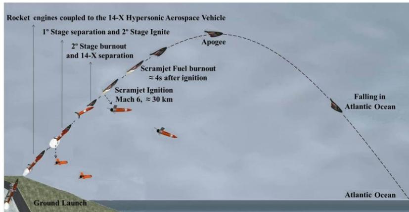
Figure 5: Hypersonic Accelerator Vehicle and VHA 14-X B in ballistic trajectory.
