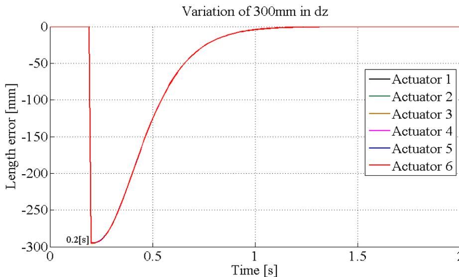
Figure 5 – Variation error in the length's actuator
