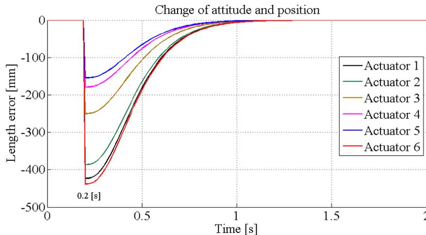
Figure 9 - Length error for a variation of attitude and position
