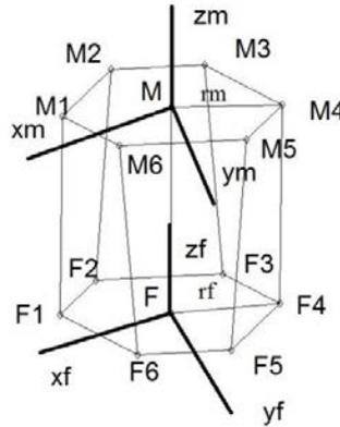
Figure 2 - Coordinate systems for fixed and movable platform
