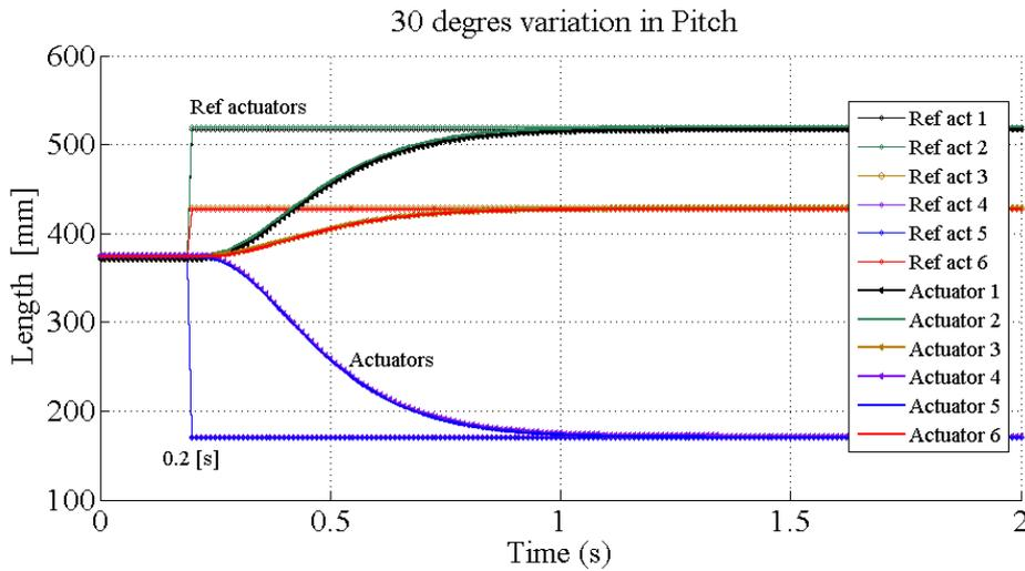
Figure 6 – Length of the actuators on the pitch variation
