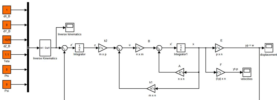
Figure 3 - The Simulink Tracking System Block Diagram
