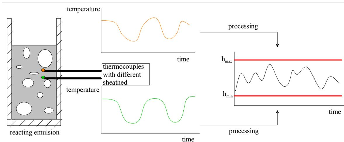
Figure 1. Strategy for monitoring of convection coefficient
