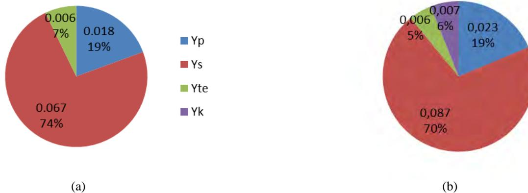
Figure 4. Loss distributions - commercial program. (a) Nozzle losses and (b) Rotor losses.
