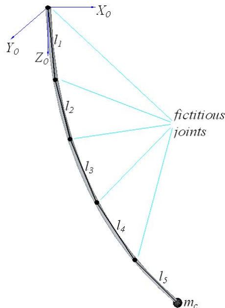
Fig. 1. Flexible structure and its discrete representation.
