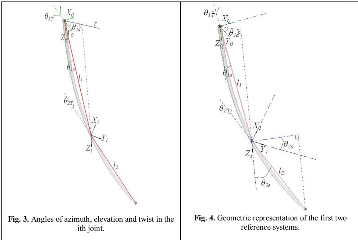
A new reference system  $(X_1Y_1Z_1)$  is incorporated into the flexible structure, centered on the second fictitious joint, as illustrated in Fig. 3, according to the convention explained previously.
