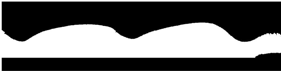
Figure 6. Image of the real interfacial wave ( $U_{ws}=0.16$  m/s and  $U_{os}=0.02$  m/s).
