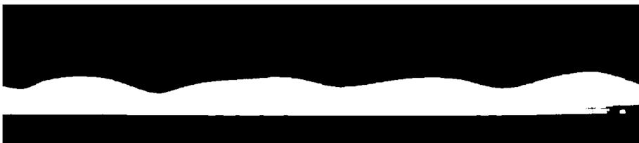
Figure 4. Image of the real interfacial wave ( $U_{ws}=0.09$  m/s and  $U_{os}=0.1$  m/s).
