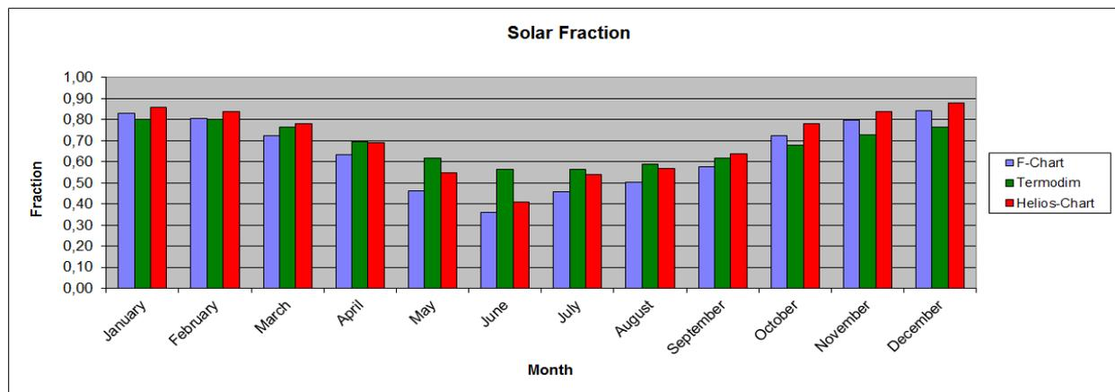
Figure 5. New comparison of solar fractions from the current software and from (Kehl, 2004)
