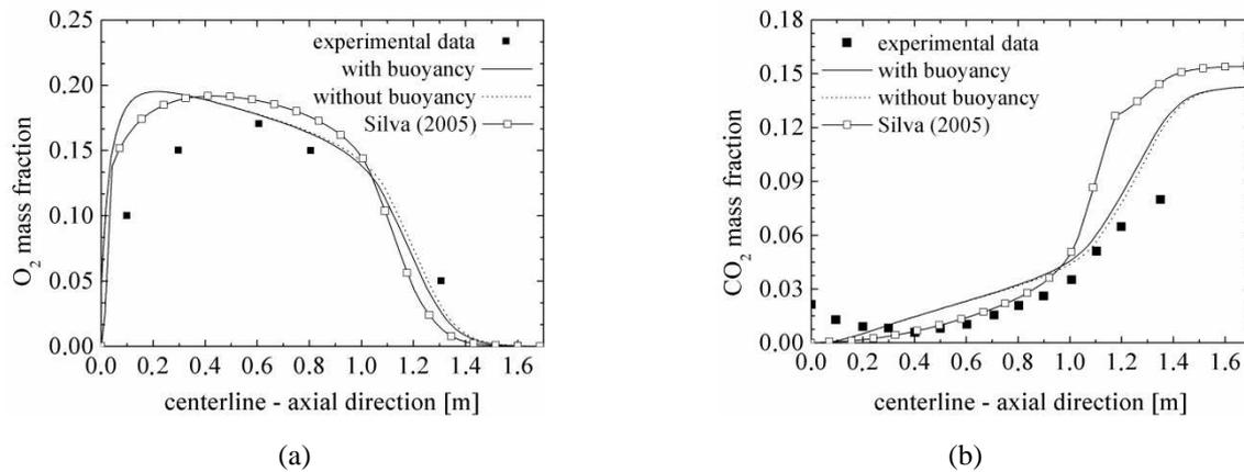
Figure 6. Mass fraction profiles at the chamber centerline: (a) O<sub>2</sub>; (b) CO<sub>2</sub>.
