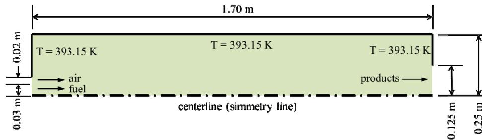
Figure 1. Combustion chamber geometry – Axisymmetric view.
