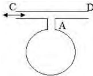
Figure 2. Closed Tube with the Helmholtz resonator in the lateral opening
