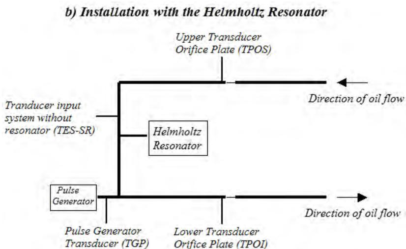
Figure 4b. Installation scheme of the bench with the main hydraulic pressure sensing assembly with the Helmholtz resonator
