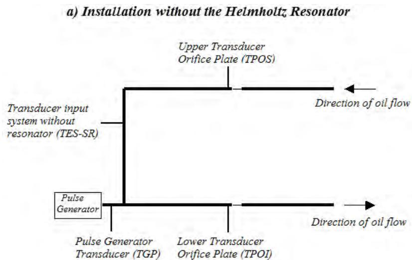
Figure 4a. Installation scheme of the bench with the main hydraulic pressure sensing assembly without the Helmholtz resonator
