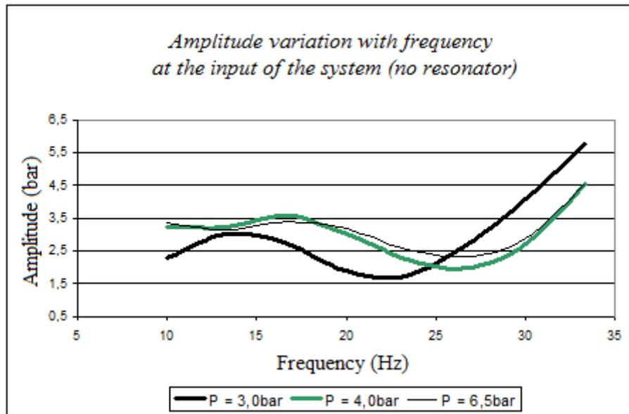
Figure 7. Variation of wave amplitude at the input of the system without resonator (TES-SR) with frequency, for different pressure levels of the hydraulic pump
