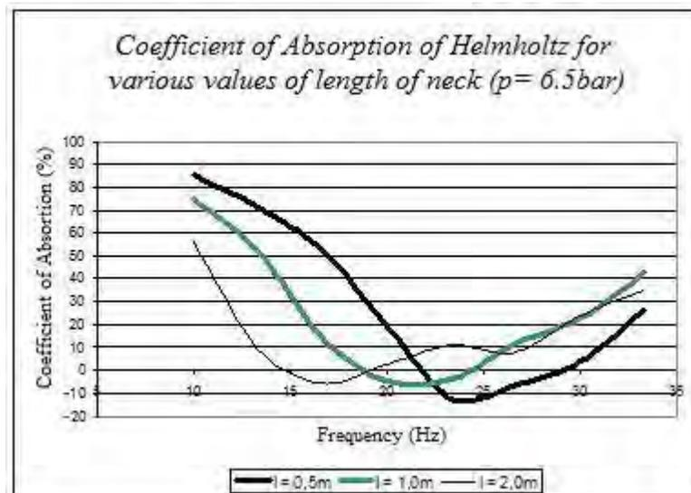
Figure 10. Absorption Coefficient of Helmholtz resonators with varying frequency, for various values of neck length and level of pressure in the system fixed at 6.5 bar
