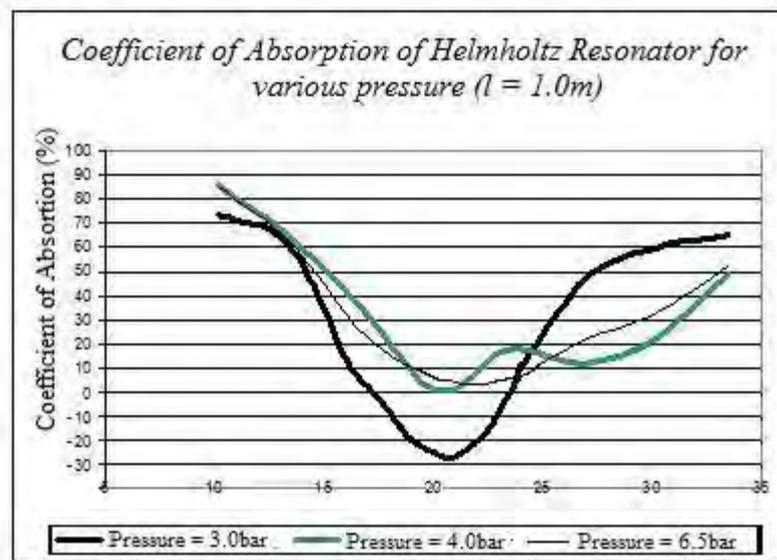
Figure 9. Absorption Coefficient of Helmholtz resonators with varying frequency, for various pressure levels and neck length set at 1.0 m
