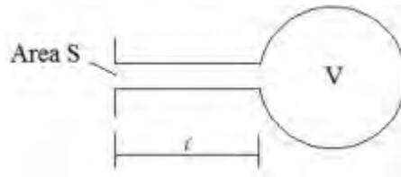
Figure 1. Simple Helmholtz Resonator
