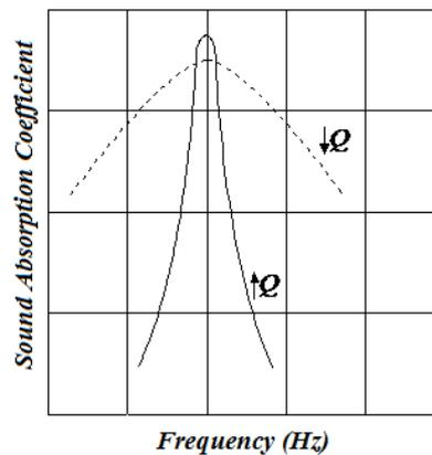
Figure 5. Sound absorption for different quality factor's Resonators Q
