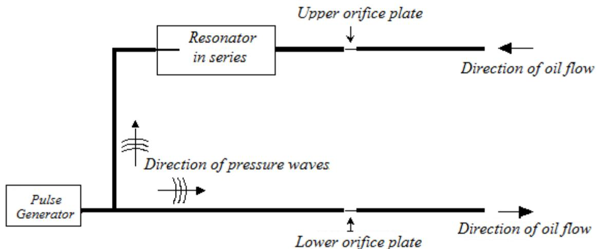
Figure 11. Schematic draw of the flow bench with the resonator in series, with the neck at the entrance of pressure waves
