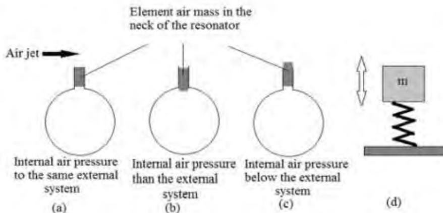
Figure 3. Analogy of the operation of the Helmholtz resonator with a mass spring system
