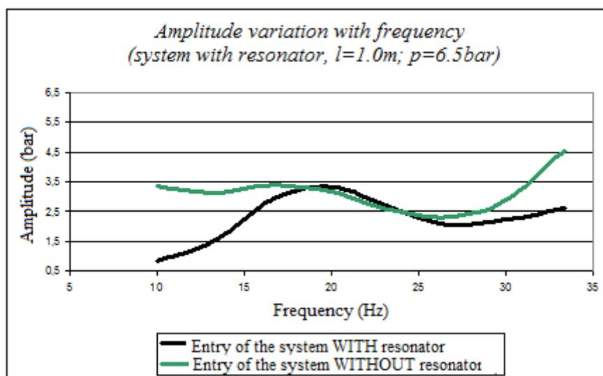
Figure 8. Variation of pressure amplitude at the input of the system with and without the Helmholtz resonator in the frequency domain, w / pressure level of 6.5 bar and 1.0 m length of the neck
