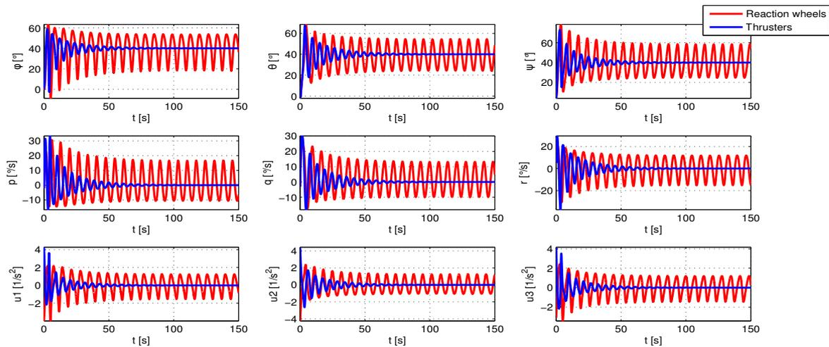
Figure 1. Close loop spacecraft response to step inputs of high amplitudes, Sarli *et al.* (2012a)
