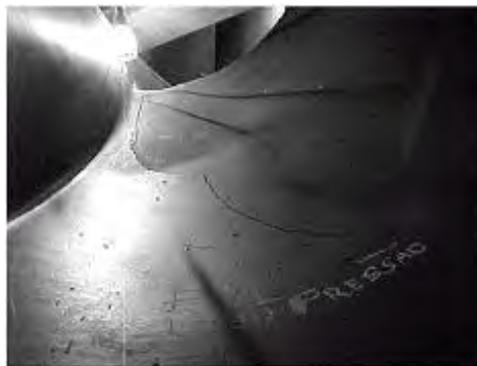
Figure 1. Crack in the blade of a hydraulic power generator.
