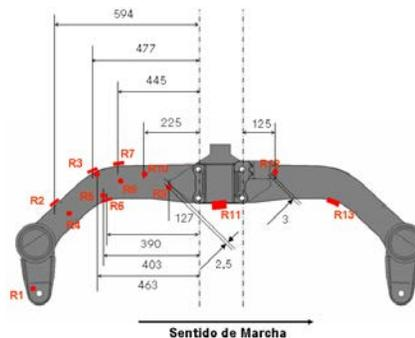
As the SSC is the current benchmark regarding structural performance and the LSC presents stresses above the yield strength in several spots, a new design is justified. Detailed strain data fatigue analysis will be conducted on the testing phase to establish damage correlation between the NSC and the SSC for precise correlation in the plastic zone.
