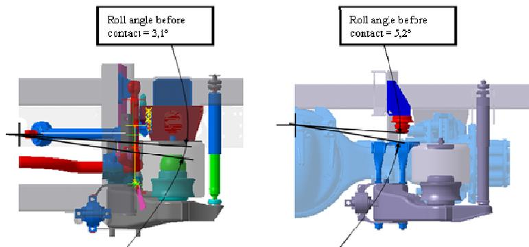
Figure 3. Vehicle lateral kinematics from CAD kinematic analysis
