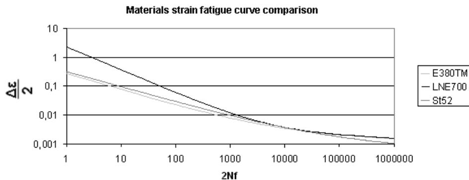
Figure 9. Experimental strain-life curves obtained for the materials
