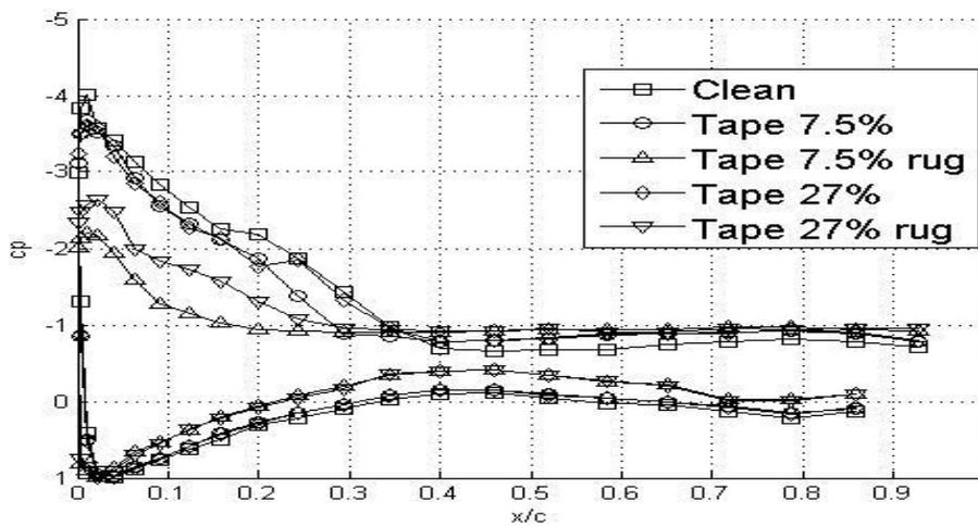
Figure 17: Curve of Cp along the chord for FFA-W3-211 and alpha = 16°.
