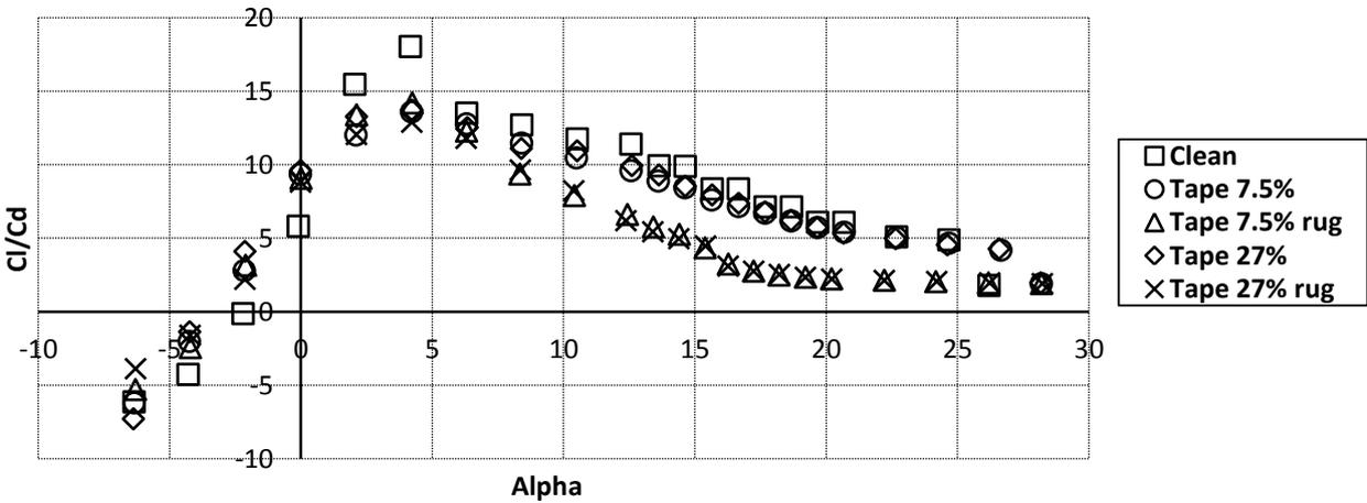
Figure 6: Comparison of the curves of Cl/Cd of the several configurations of colocation of tape and tape plus rugosity, for the DU93-W-210 airfoil.
