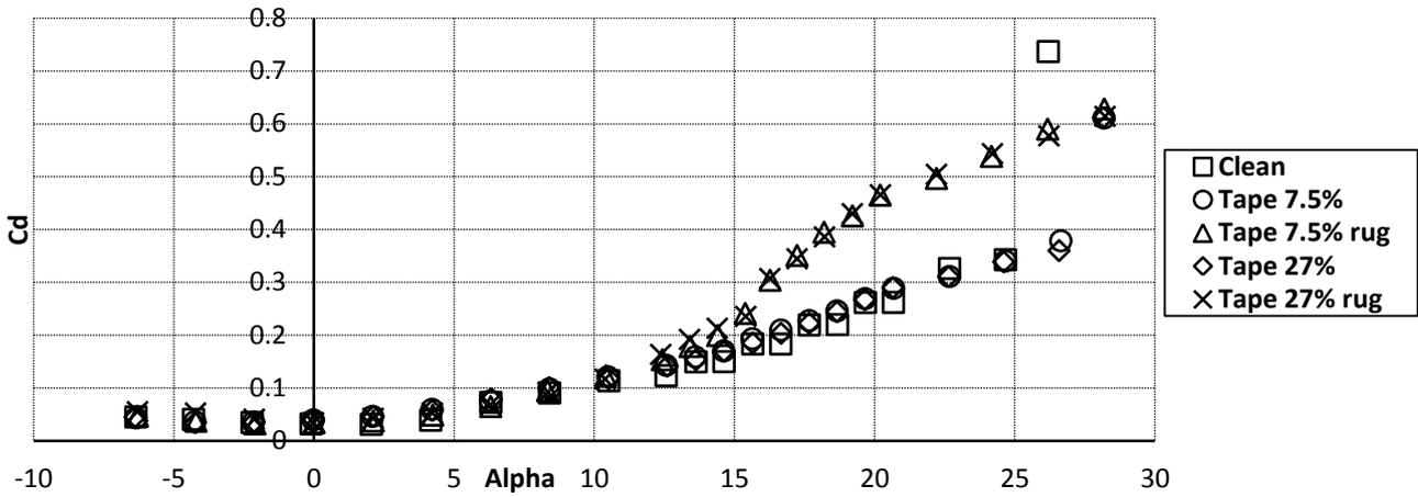
Figure 4: Comparison of the curves of Cd of the several configurations of colocation of tape and tape plus rugosity, for the DU93-W-210 airfoil.
