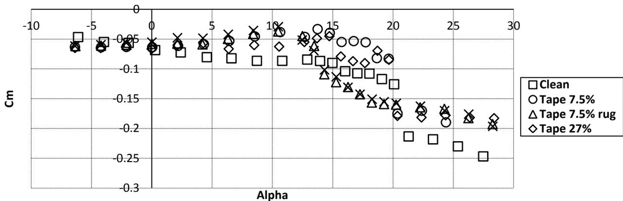
Figure 21: Comparison of the curves of  $C_m$  of the several configurations of colocation of tape and tape plus rugosity, for the NACA 63-415 airfoil.
