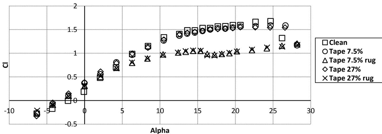
Figure 3: Comparison of the curves of  $C_l$  of the several configurations of colocation of tape and tape plus rugosity, for the DU93-W-210 airfoil
