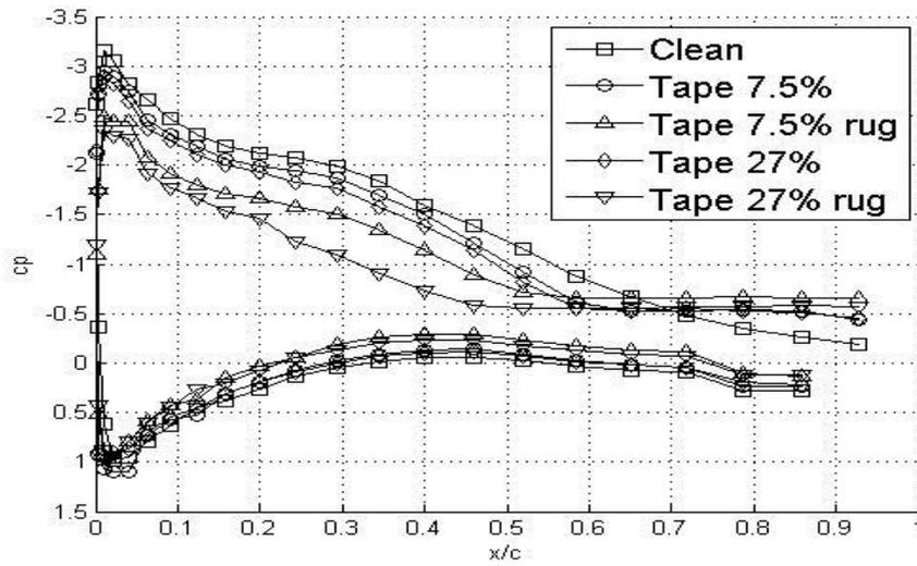
Figure 8: Curve of Cp along the chord for DU93-W-210 and alpha = 12°.
