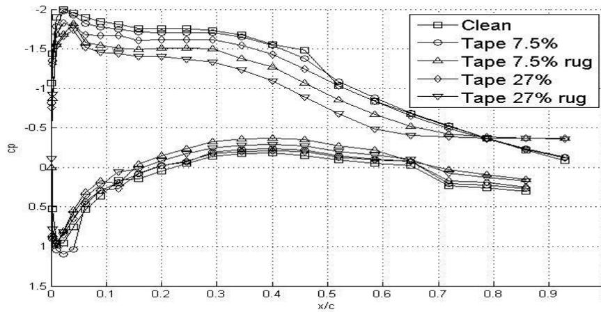
Figure 7: Curve of Cp along the chord for DU93-W-210 and alpha = 8°.
