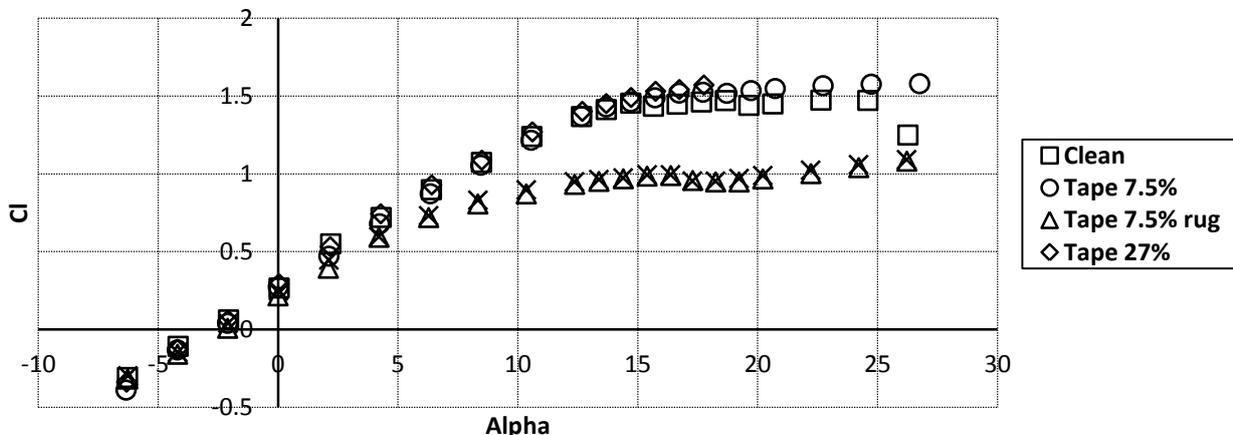
Figure 11: Comparison of the curves of  $Cl$  of the several configurations of colocation of tape and tape plus rugosity, for the FFA-W3-211 airfoil.
