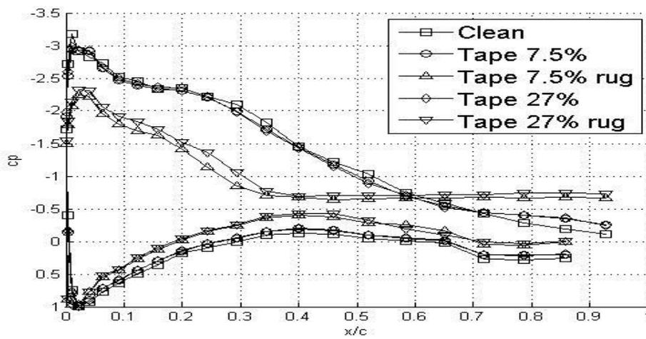
Figure 16: Curve of Cp along the chord for FFA-W3-211 and alpha = 12°.
