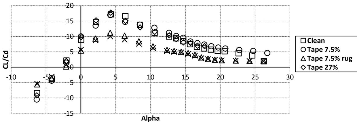
Figure 14: Comparison of the curves of Cl/Cd of the several configurations of colocation of tape and tape plus rugosity, for the FFA-W3-211 airfoil.
