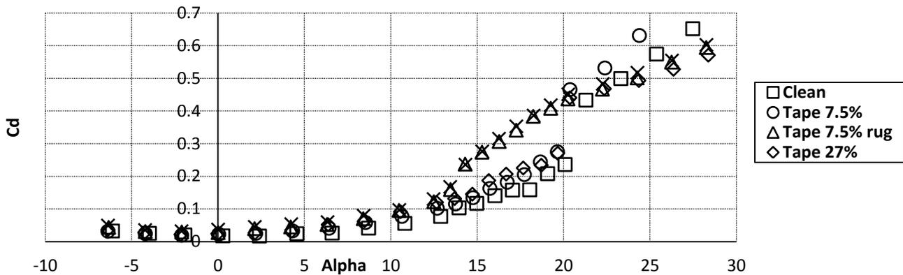
Figure 20: Comparison of the curves of  $C_d$  of the several configurations of colocation of tape and tape plus rugosity, for the NACA 63-415 airfoil.
