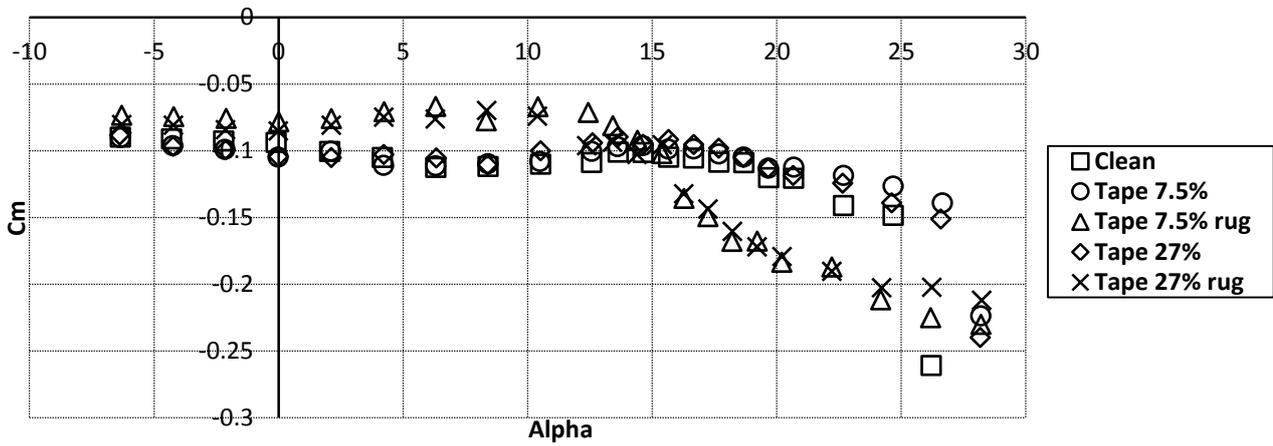
Figure 5: Comparison of the curves of Cm of the several configurations of colocation of tape and tape plus rugosity, for the DU93-W-210 airfoil.
