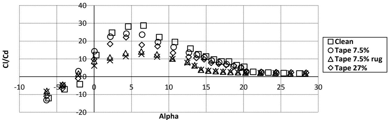
Figure 22: Comparison of the curves of  $Cl/C_d$  of the several configurations of colocation of tape and tape plus rugosity, for the NACA 63-415 airfoil.
