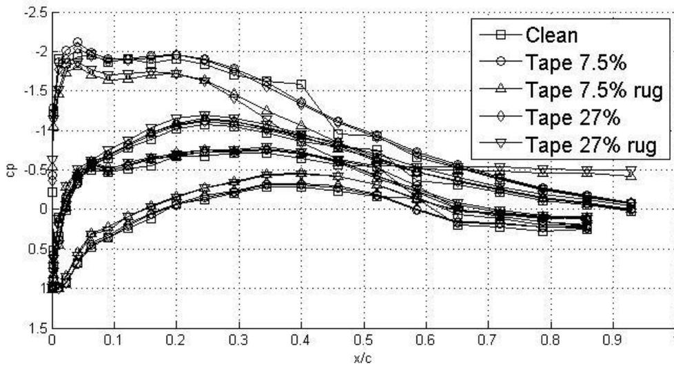
Figure 15: Curve of Cp along the chord for FFA-W3-211 and alpha = 8°.
