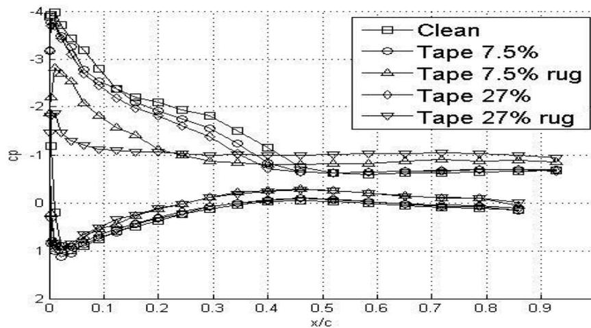
Figure 9: Curve of Cp along the chord for DU93-W-210 and alpha = 16°.
