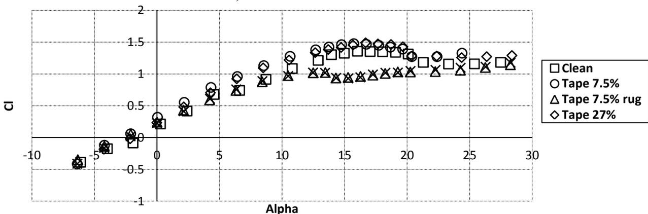
Figure 19: Comparison of the curves of  $Cl$  of the several configurations of colocation of tape and tape plus rugosity, for the NACA 63-415 airfoil.
