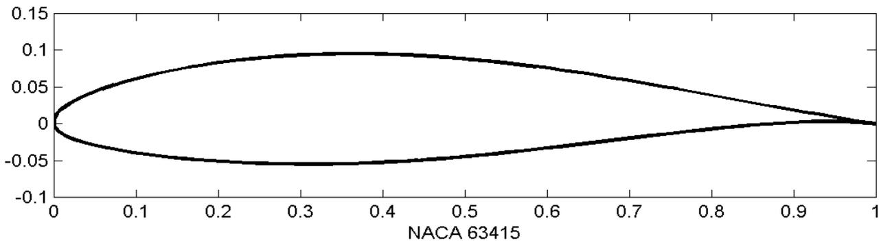
Figure 18: NACA 63415 Airfoil.
