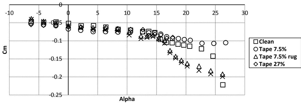
Figure 13: Comparison of the curves of Cm of the several configurations of colocation of tape and tape plus rugosity, for the FFA-W3-211 airfoil.
