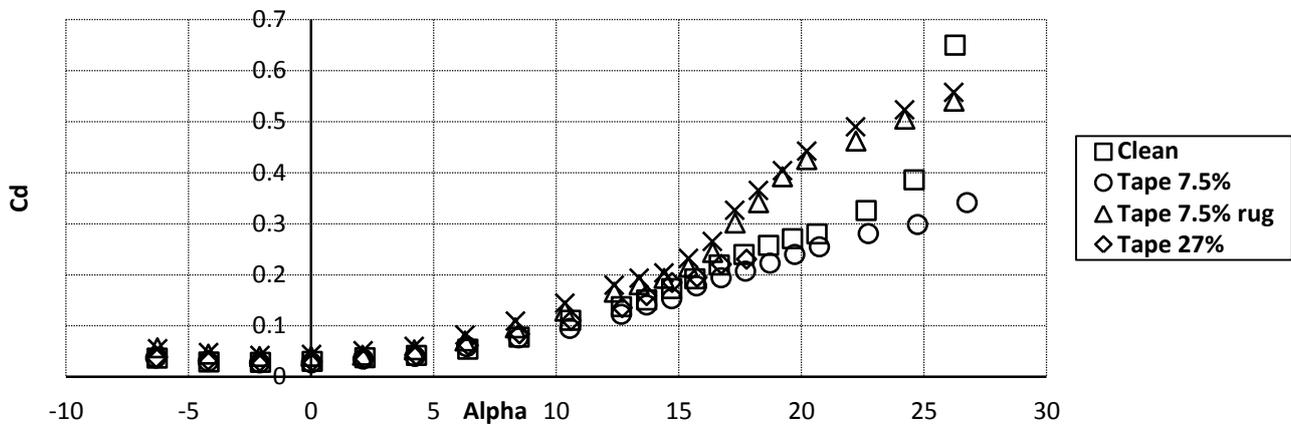
Figure 12: Comparison of the curves of Cd of the several configurations of colocation of tape and tape plus rugosity, for the FFA-W3-211 airfoil.
